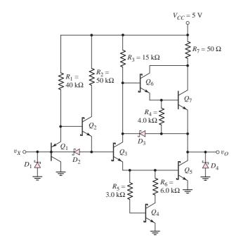
Figure 17.35 Advanced low-power Schottky (ALS) inverter gate
