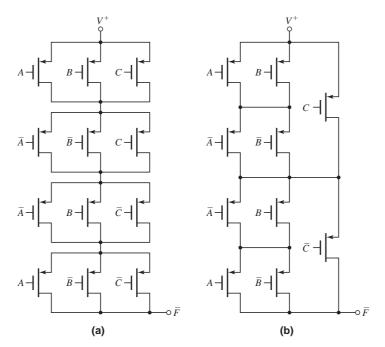
**Figure 16.97** (a) The basic PMOS pull-up portion of the logic gate derived as the complement of the basic NMOS pull-down circuit; (b) the modified PMOS pull-up portion of the logic gate for the design application
