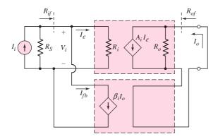
Figure 12.9 Ideal shunt-series feedback topology
