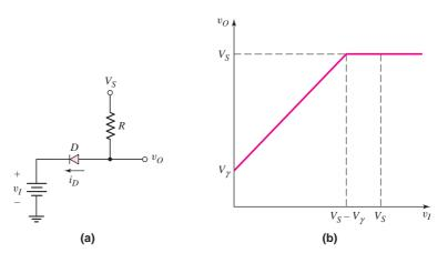
Figure 2.34 Diode with input voltage source: (a) circuit and (b) voltage transfer characteristics
