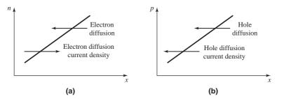
**Figure 1.9** (a) Assumed electron concentration versus distance in a semiconductor, and the resulting electron diffusion and electron diffusion current density, (b) assumed hole concentration versus distance in a semiconductor, and the resulting hole diffusion and hole diffusion current density
