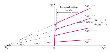
Figure 5.14 Current-voltage characteristics for the common-emitter circuit, showing the Early voltage and the finite output resistance,  $r_o$ , of the transistor
