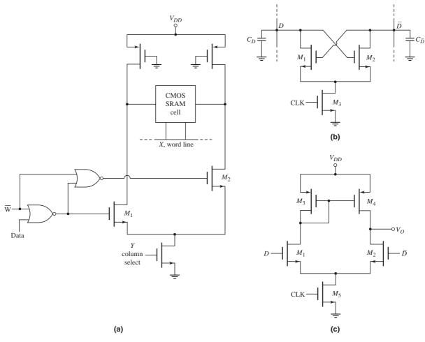
**Figure 16.80** (a) Write circuitry associated with CMOS RAM cell; (b) cross-coupled NMOS sense amplifier; (c) CMOS differential sense amplifier
