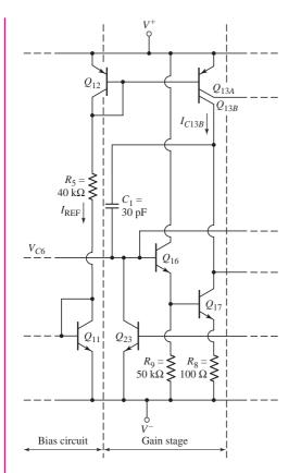
Figure 13.7 Reference circuit and gain stage, 741 op-amp
