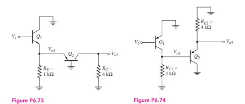
6.74 The transistor parameters in the ac equivalent circuit shown in Figure P6.74 are  $\beta_1 = \beta_2 = 100$ ,  $V_{A1} = V_{A2} = \infty$ ,  $I_{CQ1} = 0.5$  mA, and  $I_{CQ2} = 2$  mA.
