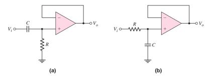
**Figure 15.3** (a) High-pass filter with voltage follower and (b) low-pass filter with voltage follower
