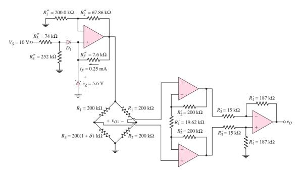
Figure 9.45 Complete amplifier system
