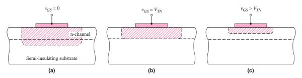
**Figure 3.58** Channel space-charge region of an enhancement-mode MESFET for: (a)  $v_{GS} = 0$ , (b)  $v_{GS} = V_{TN}$ , and (c)  $v_{GS} > V_{TN}$
