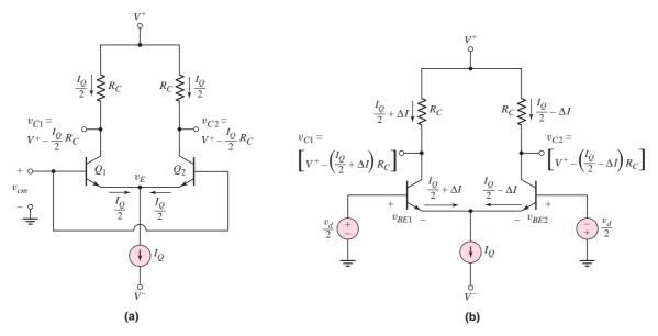
Figure 11.3 Basic diff-amp with applied common-mode voltage and (b) basic diff-amp with applied differential-mode voltage
