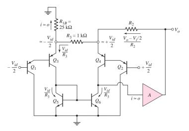
Figure 15.43 The ac equivalent circuit, LM380 power amplifier
