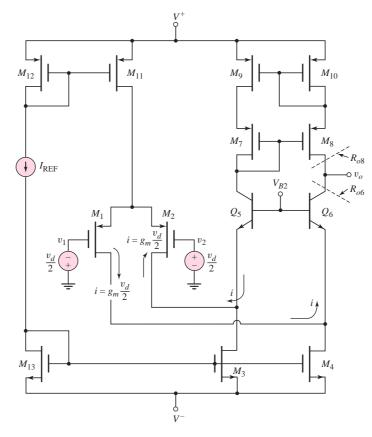
Figure 13.20 BiCMOS folded cascode amplifier
