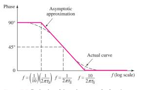
**Figure 7.7** Bode plot of the voltage transfer function phase for the circuit in Figure 7.2
