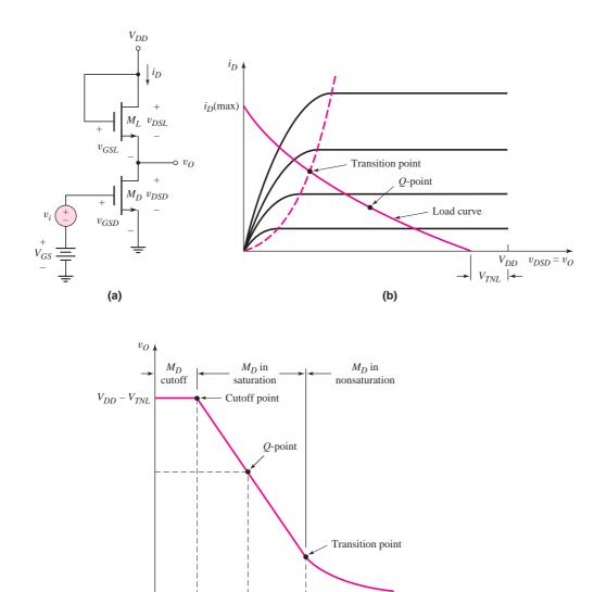
**Figure 4.39** (a) NMOS amplifier with enhancement load device; (b) driver transistor characteristics and enhancement load curve with transition point; and (c) voltage transfer characteristics of NMOS amplifier with enhancement load device
