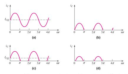
**Figure 8.15** Collector current versus time characteristics: (a) class-A amplifier, (b) class-B amplifier, (c) class-AB amplifier, and (d) class-C amplifier
