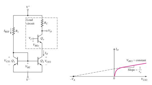
Figure 10.3 The dc equivalent circuit of simple amplifier biased with twotransistor current source
