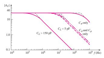
Figure 7.63 PSpice analysis results for common-base circuit
