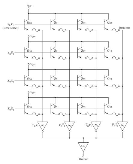
Figure 16.84 A bipolar fuse-linked user-programmable ROM
