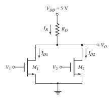
Figure 3.46 A two-input NMOS NOR logic gate
