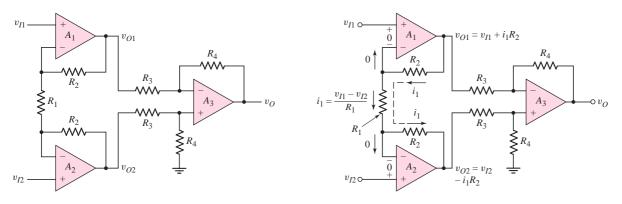
Figure 9.26 Instrumentation amplifier
