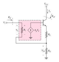
Figure 12.28 Equivalent circuit, op-amp series-series feedback configuration
