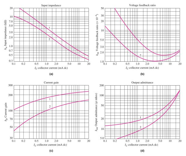
**Figure 6.21** *h*-parameter data for the 2N2222A transistor. Curves 1 and 2 represent data from high-gain and low-gain transistors, respectively.
