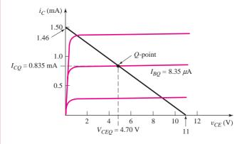
Figure 5.39 Load line and Q-point for the circuit shown in Figure 5.38(a) for Example 5.10
