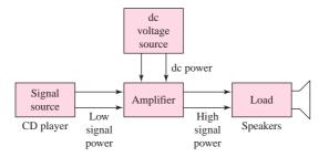
Figure PR1.1 Schematic of an electronic circuit with two input signals: the dc power supply input, and the signal input
