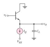
Figure 17.18 Emitterfollower stage with load capacitance
