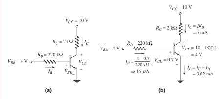
Figure 5.20 Circuit for Example 5.3: (a) circuit and (b) circuit showing current and voltage values
