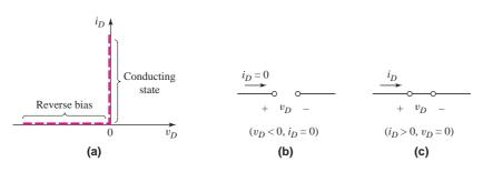
**Figure 1.26** The ideal diode: (a) the *I*–*V* characteristics of the ideal diode, (b) equivalent circuit under reverse bias (an open circuit), and (c) equivalent circuit in the conducting state (a short circuit)
