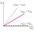
**Figure 3.8** Plot of  $i_D$  versus  $v_{DS}$  characteristic for small values of  $v_{DS}$  at three  $v_{GS}$  voltages
