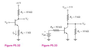
5.33 (a) The current gain of the transistor in Figure P5.33 is  $\beta = 75$ . Determine  $V_O$  for: (i)  $V_{BB} = 0$ , (ii)  $V_{BB} = 1$  V, and (iii)  $V_{BB} = 2$  V. (b) Verify the results of part (a) with a computer simulation.
