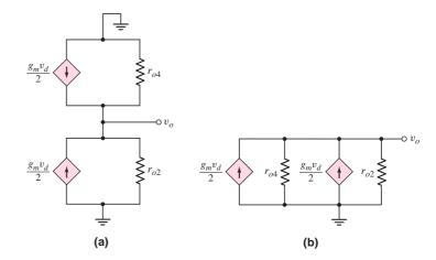
Figure 11.33 The ac equivalent circuit, MOSFET differential amplifier with active load
