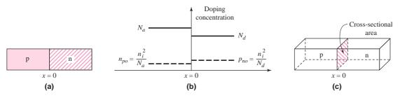
**Figure 1.10** (a) The pn junction: (a) simplified one-dimensional geometry, (b) doping profile of an ideal uniformly doped pn junction, and (c) three-dimensional representation showing the cross-sectional area
