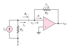
Figure 9.20 Current-to-voltage converter
