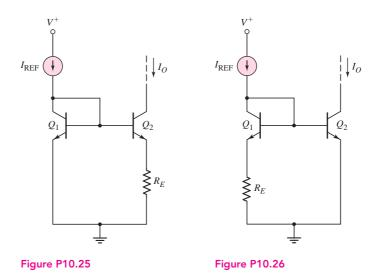
10.26 Consider the circuit in Figure P10.26. Neglect base currents and assume  $V_A = \infty$ . Assume  $I_{\text{REF}} = 100 \,\mu\text{A}$  and  $R_E = 700 \,\Omega$ . (a) For transistor parameters of  $I_{S1} = I_{S2} = 5 \times 10^{-15} \text{ A}$ , find  $V_{BE1}$ ,  $V_{BE2}$ , and  $I_O$ . (b) Repeat
