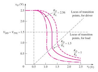
Figure 16.8 Voltage transfer characteristics of an NMOS inverter with depletion load, using parameters from Example 16.3 and for three aspect ratios
