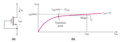
Flgure 4.42 (a) NMOS depletion-mode transistor with gate and source connected in a load device configuration and (b) current–voltage characteristic of NMOS depletion load transistor
