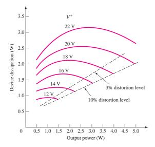
Figure 15.44 LM380 power amplifier characteristics
