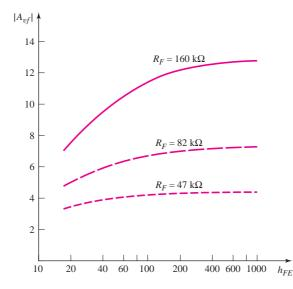
**Figure 12.38** Voltage gain magnitude versus transistor current gain, for three values of feedback resistance, from a PSpice analysis of the circuit in Figure 12.37(a)
