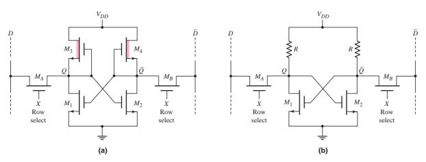
Figure 16.74 Static NMOS RAM cells with (a) depletion loads and (b) polysilicon resistor loads
