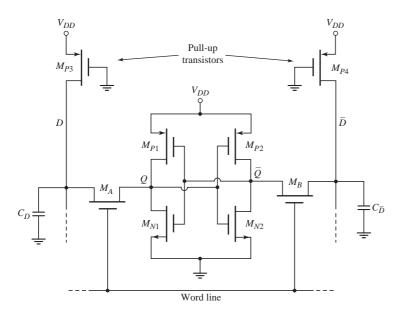
Figure 16.76 CMOS RAM cell including PMOS pull-up transistors
