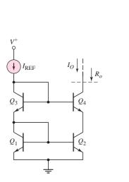
Figure 11.41 Bipolar cascode constant-current source
