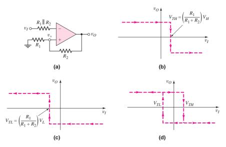
**Figure 15.28** (a) Schmitt trigger circuit, (b) voltage transfer characteristic as input voltage increases, (c) voltage transfer characteristic as input voltage decreases, and (d) net voltage transfer characteristics, showing hysteresis effect
