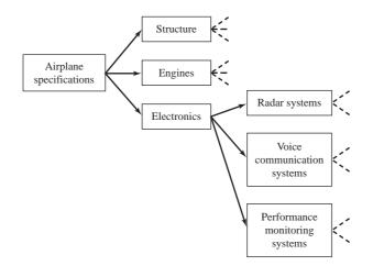
Figure PR2.2 System and subsystem block diagrams for an airplane
