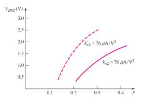
Figure 14.32 Change in drain-to-source voltage as the compensation network is varied
