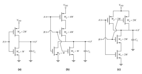
Figure 16.36 The width-to-length ratios of (a) the CMOS inverter, (b) the CMOS NOR gate, and (c) the CMOS NAND gate
