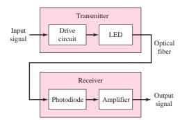
Figure 1.40 Basic elements in an optical transmission system
