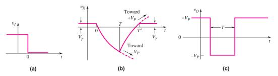
**Figure 15.38** Schmitt trigger monostable multivibrator voltages versus time (a) input trigger pulse, (b) capacitor voltage, and (c) output pulse
