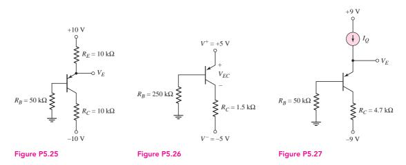
5.28 In the circuit in Figure P5.27, the constant current is I = 0.5 mA. If  $\beta = 50$ , determine the power dissipated in the transistor. Does the constant current source supply or dissipate power? What is the value?
