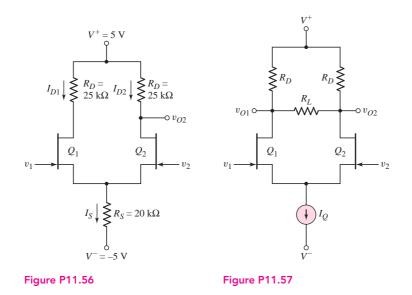
\*11.57 Consider the circuit in Figure P11.57. Assume that  $\lambda = 0$  for the transistors, and assume an ideal current source  $I_Q$ . Derive the expressions for the one-sided differential-mode gains  $A_{d1} = v_{o1}/v_d$  and  $A_{d2} = v_{o2}/v_d$ , and for the two-sided differential-mode gain  $A_d = (v_{o2} - v_{o1})/v_d$ .
