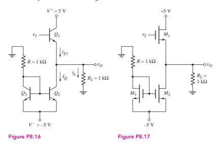
8.17 Consider the class-A source-follower circuit shown in Figure P8.17. The transistors are matched with parameters  $V_{TN} = 0.5$  V,  $K_n = 12$  mA/V<sup>2</sup>, and  $\lambda = 0$ . Determine the maximum and minimum values of output voltage
