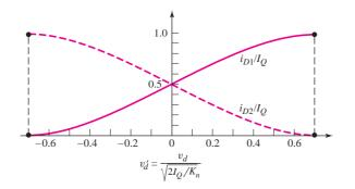
Figure 11.21 Normalized dc transfer characteristics, MOSFET differential amplifier
