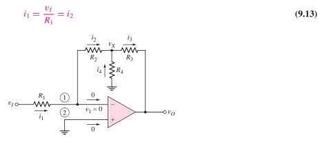
Figure 9.12 Inverting op-amp with T-network
