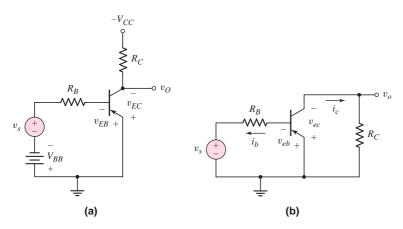
Figure 6.14 (a) A common-emitter circuit with a pnp transistor and (b) the corresponding ac equivalent circuit
