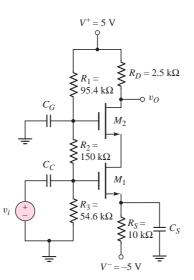
Figure 4.51 NMOS cascode circuit
