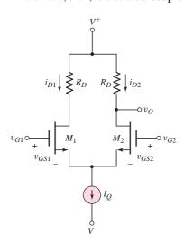
Figure 11.19 Basic MOSFET differential pair configuration
