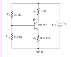
Figure 5.56 PSpice circuit schematic for Design Example 5.16
