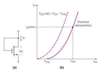
Figure 4.38 (a) NMOS enhancement-mode transistor with gate and drain connected in a load device configuration and (b) current–voltage characteristics of NMOS enhancement load transistor
