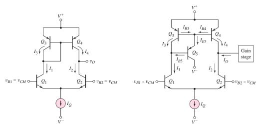
Figure 11.28 BJT differential amplifier with active load
