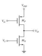
Figure 3.41 Example of CMOS inverter
