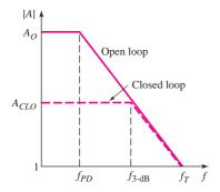
Figure 14.10 Bode plot, open-loop and closed-loop gain magnitude
