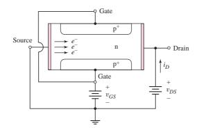
Figure 3.54 Cross section of a symmetrical n-channel pn junction field-effect transistor
