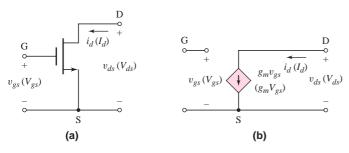
Figure 4.5 (a) Common-source NMOS transistor with small-signal parameters and (b) simplified small-signal equivalent circuit for NMOS transistor
