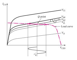
Figure 10.31 Driver transistor characteristics and load curve for BJT circuit with active load
