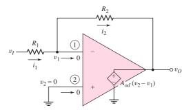
Figure 9.9 Inverting op-amp equivalent circuit
