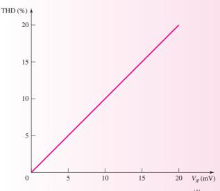
**Figure 6.6** Total harmonic distortion of the function  $e^{v_{BE}/V_T}$ , where  $v_{BE} = V_{\pi} \sin \omega t$ , as a function of  $V_{\pi}$
