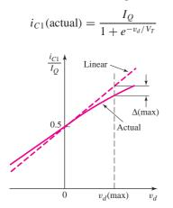
Figure 11.6 Expanded view, normalized  $i_{C1}$  versus  $v_d$  transfer characteristic
