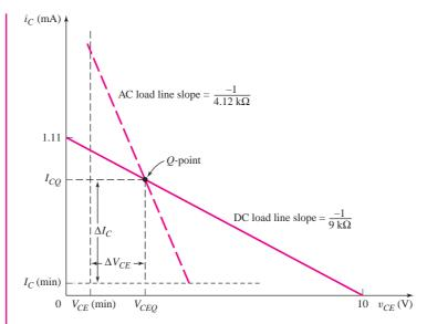
**Figure 6.47** The ac and dc load lines to find the maximum symmetrical swing for the circuit shown in Figure 6.46(a) used in Example 6.11
