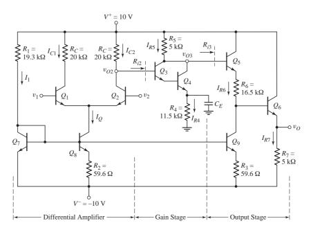
Figure 11.49 Bipolar operational amplifier circuit
