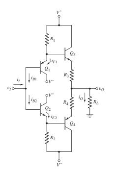
Figure 8.34 Class-AB output stage with input buffer transistors
