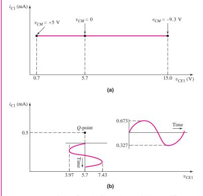
**Figure 11.4** (a) Variation of *Q*-point for transistor  $Q_1$  in the BJT diff-amp as the commonmode input voltage varies from +5 to -9.3 V; (b) change in collector current and collector–emitter voltage versus time for transistor  $Q_1$  in the BJT diff-amp when a sinusoidal 18 mV differential voltage is applied
