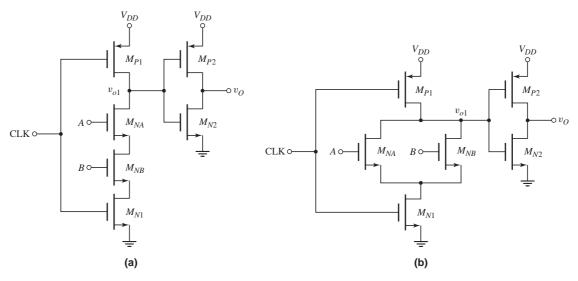
Figure 16.44 Clocked CMOS logic circuit: (a) AND function and (b) OR function
