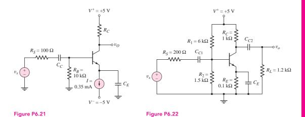
6.22 For the circuit in Figure P6.22, the transistor parameters are  $\beta = 180$  and  $r_o = \infty$ . (a) Determine the *Q*-point values. (b) Find the small-signal hybrid- $\pi$  parameters. (c) Find the small-signal voltage gain  $A_v = v_o/v_s$ .
