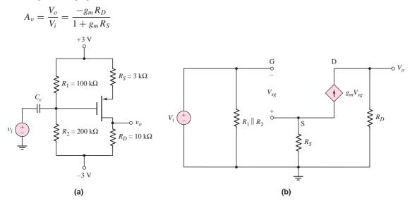
Figure 4.20 (a) PMOS circuit for Example 4.5, and (b) small-signal equivalent circuit
