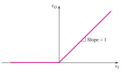
Figure 9.34 Voltage transfer characteristics of precision half-wave rectifier
