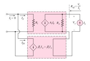
Figure 12.10 Ideal shunt-series feedback configuration for determining output resistance
