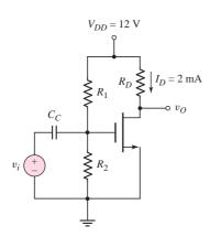
Figure 4.17 Common-source NMOS transistor circuit
