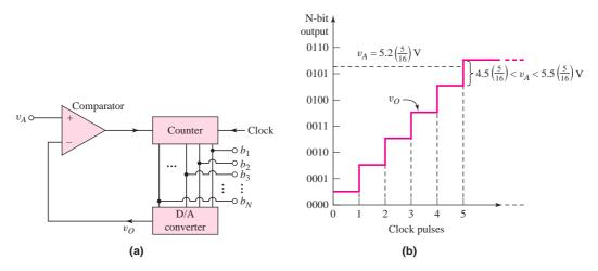
**Figure 16.94** (a) Block diagram of a counting A/D converter and (b) the timing diagram of a 4-bit A/D counting converter for a specific input voltage
