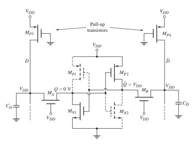
Figure 16.77 Voltage levels and "on" transistors in CMOS RAM cell at the beginning of the read cycle
