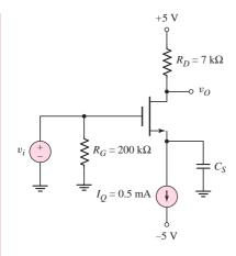
Figure 4.21 NMOS common-source circuit with source bypass capacitor
