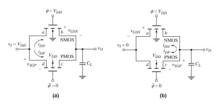
Figure 16.57 Currents and gate–source voltages in CMOS transmission gate for: (a) input high condition and (b) input low condition
