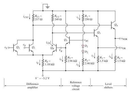
Figure 17.5 Basic ECL logic gate with reference circuit
