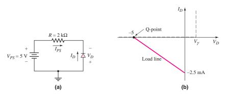
Figure 1.33 Reverse-biased diode (a) circuit and (b) piecewise linear approximation and load line
