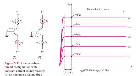
Figure 5.12 Transistor current–voltage characteristics of the common-base circuit
