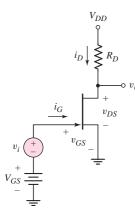
Figure 4.53 JFET commonsource circuit with timevarying signal source in series with gate dc source
