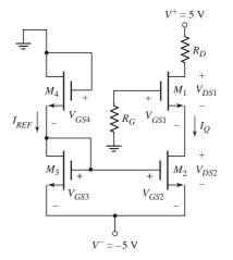
Figure 3.50 Implementation of a MOSFET constant-current source
