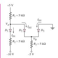
Figure 2.40 Diode circuit for Example 2.11
