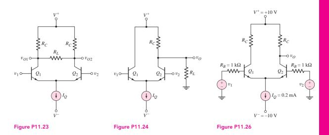
expressions for the one-sided differential-mode gain  $A_{v1} = v_{o1}/v_d$  and  $A_{v2} = v_{o2}/v_d$ , and for the two-sided differential-mode gain  $A_d = (v_{o2} - v_{o1})/v_d$ .
