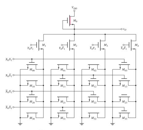
Figure 16.83 An NMOS  $16 \times 1$  mask-programmable ROM
