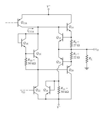
Figure 13.9 Output stage, 741 op-amp with short-circuit protection devices
