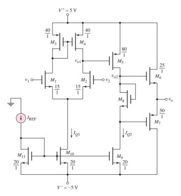
Figure 13.15 A three-stage CMOS operational amplifier
