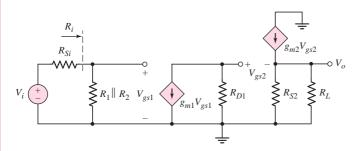
Figure 4.50 Small-signal equivalent circuit of NMOS cascade circuit
