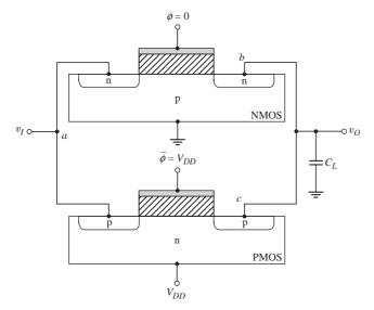
Figure 16.58 CMOS transmission gate showing cross sections of NMOS and PMOS transistors
