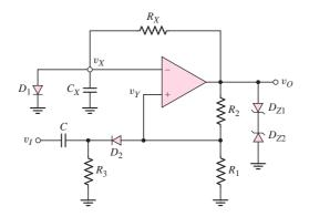
Figure 15.37 Schmitt trigger monostable multivibrator
