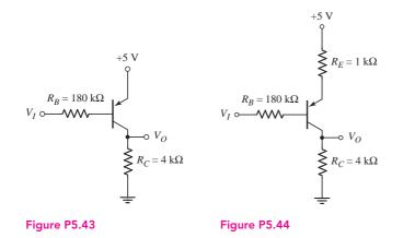
5.44 For the circuit shown in Figure P5.44, plot the voltage transfer characteristics over the range  $0 \le V_I \le 5$  V. Assume  $\beta = 100$ .
