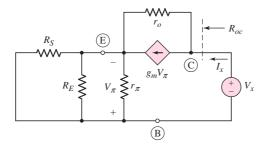
Figure 6.62 Common-base equivalent circuit for output resistance calculations
