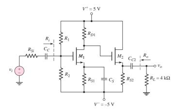
Figure 3.52 Common-source amplifier in cascade with source follower
