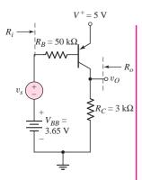
Figure 6. 18 pnp commonemitter circuit for Example 6.3
