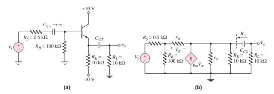
**Figure 7.23** (a) Emitter-follower circuit with output coupling capacitor and (b) small-signal equivalent circuit
