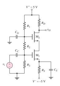
Figure 3.53 NMOS cascode circuit
