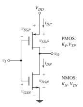
Figure 16.21 CMOS inverter
