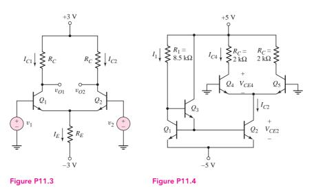
11.4 The differential amplifier in Figure P11.4 is biased with a three-transistor current source. The transistor parameters are:  $\beta = 100$ ,  $V_{BE}(\text{on}) = 0.7$  V, and
