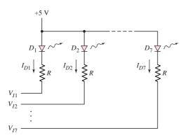
Figure 2.46 Control circuit for the seven-segment LED display
