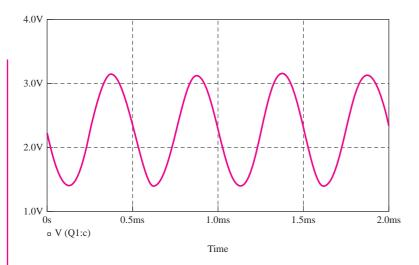
**Figure 5.49** Output signal from the circuit shown in Figure 5.48 for input signals of  $V_{BB} = 1.3$  V and  $\Delta v_I = 0.2 \sin \omega t$  (V)
