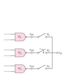
Figure 17.28 Circuit symbolically showing tristate output
