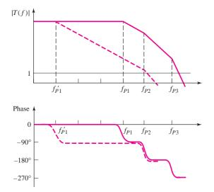
**Figure 12.61** Bode plots of loop gain for three-stage amplifier, before (solid curves) and after (dotted curves) incorporating Miller compensation capacitor: (a) magnitude and (b) phase
