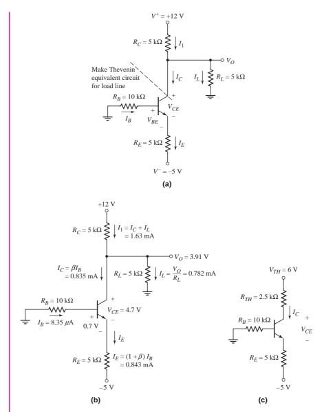
**Figure 5.38** Circuit for Example 5.10: (a) circuit; (b) circuit showing current and voltage values; and (c) Thevenin equivalent circuit
