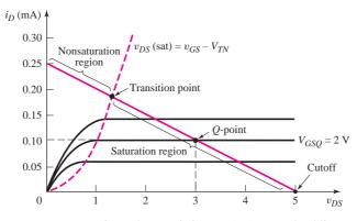
Figure 3.31 Transistor characteristics,  $v_{DS}(\text{sat})$  curve, load line, and *Q*-point for the NMOS common-source circuit in Figure 3.25(b)
