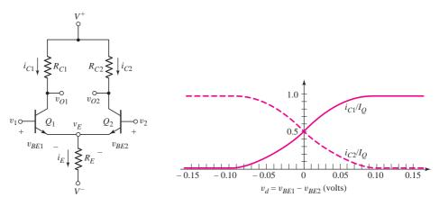
Figure 17.1 Basic differential amplifier circuit
