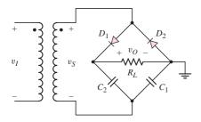
Figure 2.14 A voltage doubler circuit
