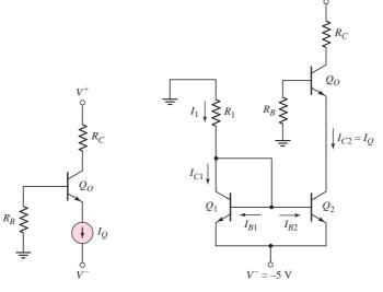
Figure 5.59 Bipolar transistor biased with a constant-current source
