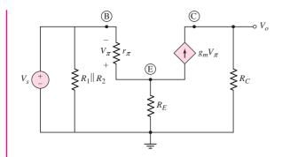
**Figure 6.33** Small-signal equivalent circuit for circuit shown in Figure 6.32(a) used in Example 6.6
