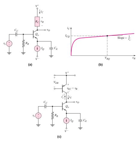
**Figure 6.40** (a) A common-emitter circuit with current source biasing and a nonlinear load resistor, (b) current–voltage characteristics of the nonlinear load resistor, and (c) pnp transistor that can be used to generate the nonlinear load characteristics
