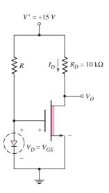
Figure 3.69 Design application circuit to measure output voltage of diode versus temperature
