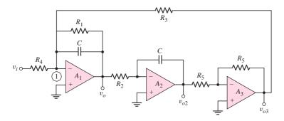
Figure 15.53 Bandpass filter network for the design application
