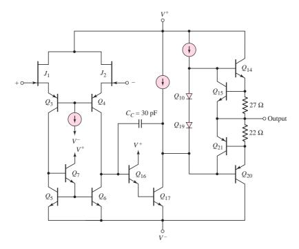
Figure 13.24 Equivalent circuit, LH0022/42/52 series hybrid JFET op-amp
