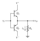
Figure 8.19 Basic complementary push–pull output stage
