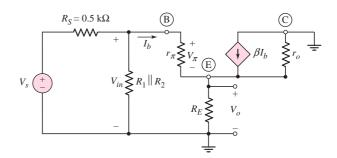
Figure 6.50 Small-signal equivalent circuit of the emitterfollower
