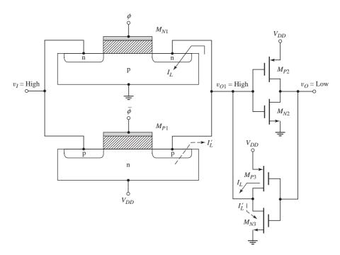
Figure 16.65 CMOS D-type flip-flop
