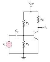
Figure 10.28 Bipolar common-emitter circuit
