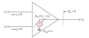
Figure 9.6 Parameters of the ideal op-amp
