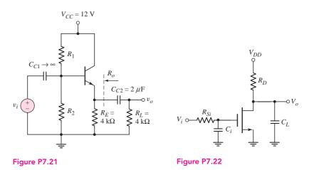
7.22 (a) For the circuit shown in Figure P7.22, write the voltage transfer function  $T(s) = V_o(s)/V_i(s)$ . Assume  $\lambda > 0$  for the transistor. (b) What is the expression for the time constant associated with the input portion of the circuit? (c) What is the expression for the time constant associated with the output portion of the circuit?
