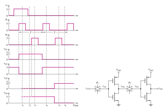
Figure 16.61 NMOS shift register voltages at various times
