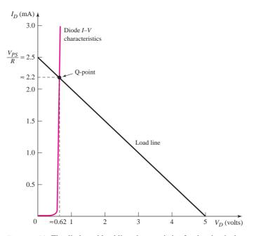
Figure 1.29 The diode and load line characteristics for the circuit shown in Figure 1.28
