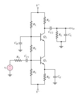
Figure 7.65 Cascode circuit
