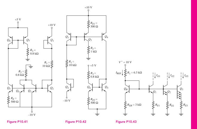
\*D10.43 Consider the circuit in Figure P10.43. The transistor parameters are:  $\beta = \infty$ ,  $V_A = \infty$ , and  $V_{BE} = 0.7$  V. Design the circuit such that the B–E voltages of  $Q_1$ ,  $Q_2$ , and  $Q_3$  are identical to that of  $Q_R$ . What are the values of  $I_{O1}$ ,  $I_{O2}$ , and  $I_{O3}$ ?
