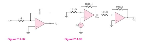
14.38 In the circuit in Figure P14.38, the offset voltage of each op-amp is ±3 mV.
