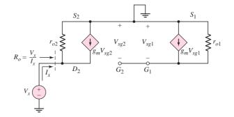
Figure 10.39 Small-signal equivalent circuit of the MOSFET active load circuit
