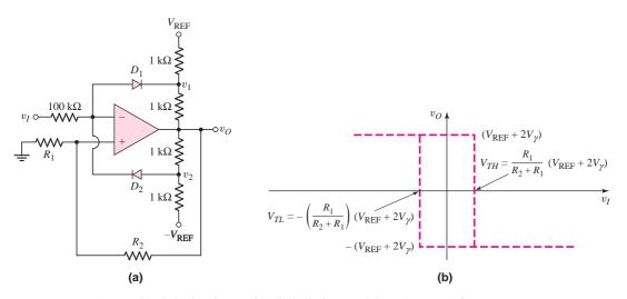
Figure 15.34 (a) Inverting Schmitt trigger with diode limiters and (b) voltage transfer characteristics
