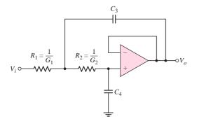
Figure 15.6 General two-pole low-pass filter
