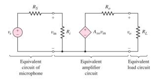
Figure 6.25 Equivalent preamplifier circuit
