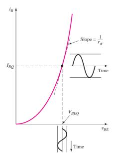
**Figure 6.5** Base current versus base–emitter voltage characteristic with superimposed sinusoidal signals. Slope at the *Q*-point is inversely proportional to  $r_{\pi}$ , a small-signal parameter.
