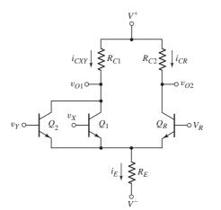
Figure 17.3 Basic two-input ECL OR/NOR logic circuit
