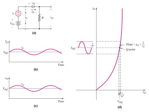
**Figure 1.35** AC circuit analysis: (a) circuit with combined dc and sinusoidal input voltages, (b) sinusoidal diode current superimposed on the quiescent current, (c) sinusoidal diode voltage superimposed on the quiescent value, and (d) forward-biased diode I-V characteristics with a sinusoidal current and voltage superimposed on the quiescent values
