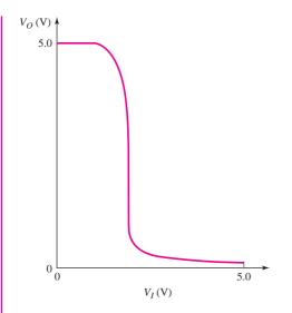
Figure 3.40 Voltage transfer characteristics of NMOS inverter with depletion load device
