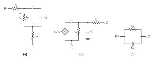
Figure 7.36 Components of the hybrid- $\pi$  equivalent circuit: (a) base to emitter, (b) collector to emitter, and (c) base to collector
