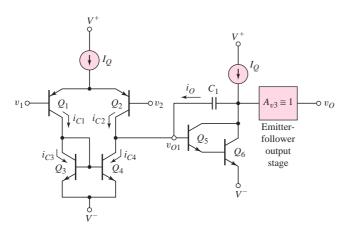
Figure 14.11 Simplified op-amp for calculating slew rate
