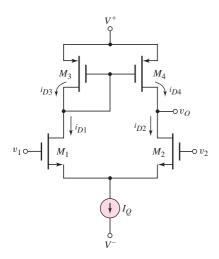
Figure 11.32 MOSFET differential amplifier with active load
