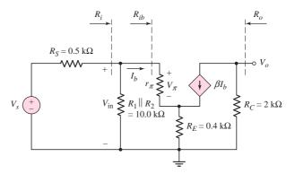
Figure 6.28 An npn common-emitter circuit with an emitter resistor, a voltage-divider biasing circuit, and a coupling capacitor
