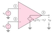
Figure 9.2 Ideal op-amp equivalent circuit
