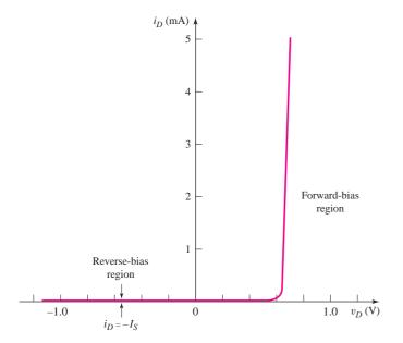
**Figure 1.17** Ideal *I*–*V* characteristics of a pn junction diode for  $I_S = 10^{-14}$  A. The diode current is an exponential function of diode voltage in the forward-bias region and is very nearly zero in the reverse-bias region. The pn junction diode is a nonlinear electronic device.
