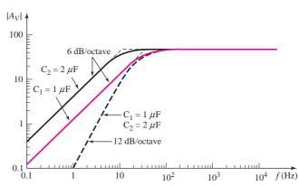
Figure 7.31 PSpice results for each coupling capacitor, and the combined effect for the circuit in Figure 7.30 ( $C_E \rightarrow \infty$ )
