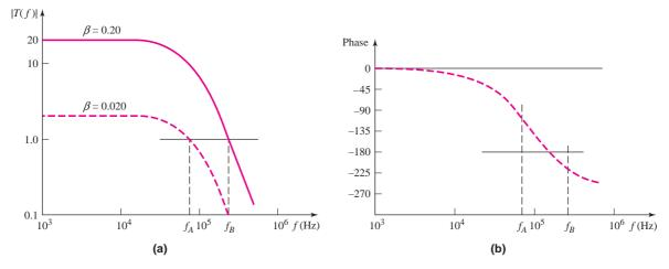
**Figure 12.56** Bode plots of loop gain of function described in Example 12.18, for two values of feedback transfer function: (a) magnitude and (b) phase
