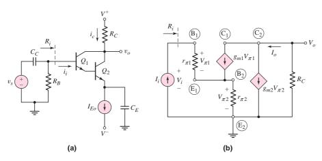
Figure 6.70 (a) A Darlington pair configuration; (b) small-signal equivalent circuit
