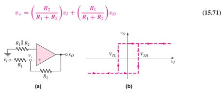
Figure 15.29 (a) Noninverting Schmitt trigger circuit and (b) voltage transfer characteristics
