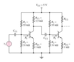
Figure 7.73 Two-stage BJT amplifier with coupling capacitors for design application
