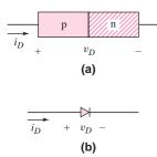
Figure 1.19 The basic pn junction diode: (a) simplified geometry and (b) circuit symbol, and conventional current direction and voltage polarity
