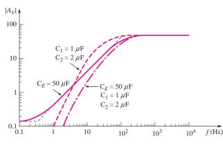
Figure 7.32 PSpice results for the two coupling capacitors, the bypass capacitor, and the combined effects
