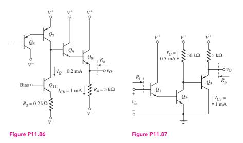
Determine the input resistance  $R_i$ , the output resistance  $R_o$ , and the small-signal voltage gain  $A_v = v_o/v_{in}$ .
