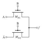
Figure 16.52 Simple NMOS pass logic network
