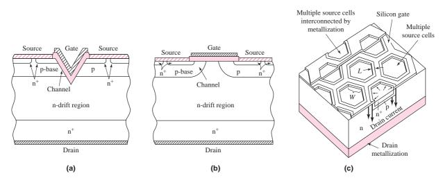
**Figure 8.8** (a) Cross section of a VMOS device; (b) cross section of DMOS device; (c) HEXFET structure
