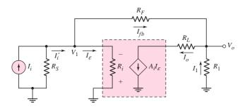
Figure 12.21 Equivalent circuit, op-amp shunt-series feedback configuration
