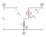
**Figure 7.51** Simplified low-frequency equivalent circuit of the n-channel common-source MOSFET including source resistance  $r_s$  but not resistance  $r_o$
