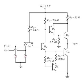
Figure 17.33 Schottky TTL NAND logic circuit
