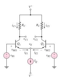
Figure 11.2 Basic BJT differential-pair configuration
