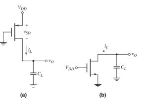
Figure 16.29 CMOS inverter when the output switches (a) low to high and (b) high to low
