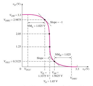
Figure 16.32 CMOS inverter voltage transfer characteristics with defined noise margins
