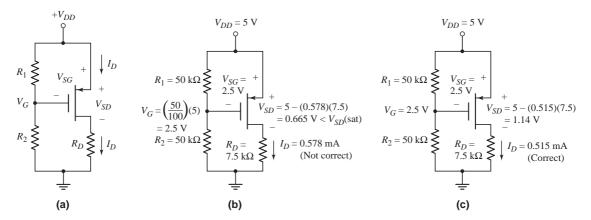
**Figure 3.26** (a) A PMOS common-source circuit, (b) the PMOS common-source circuit for Example 3.4 showing current and voltage values when the saturation-region bias assumption is incorrect, and (c) the circuit for Example 3.4 showing current and voltage values when the nonsaturation-region bias assumption is correct
