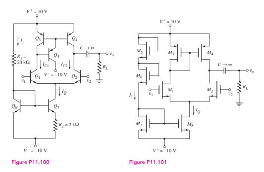
11.101 Consider the circuit in Figure P11.101. Use standard transistors. Using a computer simulation, determine the small-signal differential-mode voltage gain and common-mode voltage gain for (a)  $R_L = 10 \text{ M}\Omega$  and (b)  $R_L = 200 \text{ k}\Omega$ .
