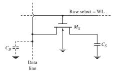
Figure 16.81 One-transistor dynamic RAM cell
