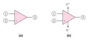
Figure 9.1 (a) Small-signal circuit symbol of the op-amp; (b) op-amp with positive and negative supply voltages
