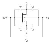
Figure 16.2 n-channel MOSFET and device capacitances
