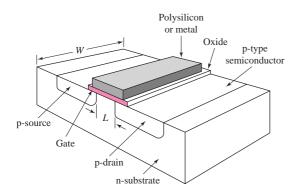
Figure 16.20 Simplified cross section of p-channel MOSFET
