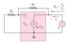
Figure 9.5 Equivalent circuit determining output resistance
