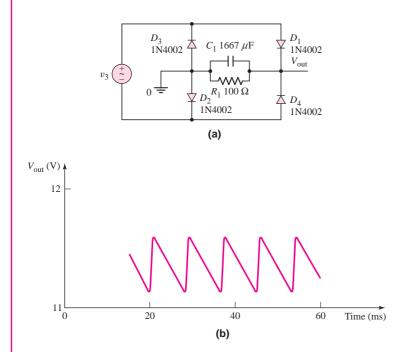
**Figure 2.12** (a) PSpice circuit schematic of diode bridge circuit with an RC filter; (b) Steady-state output voltage of PSpice analysis of diode bridge circuit for a 60 Hz input sine wave with a peak value of 13.4 V
