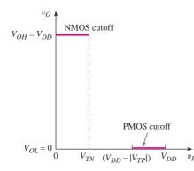
Figure 16.24 CMOS inverter output voltage for input voltage in either high state or low state
