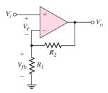
Figure 12.16 Example of an op-amp series–shunt feedback circuit
