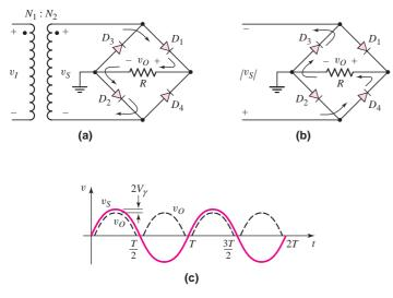
**Figure 2.6** A full-wave bridge rectifier: (a) circuit showing the current direction for a positive input cycle, (b) current direction for a negative input cycle, and (c) input and output voltage waveforms
