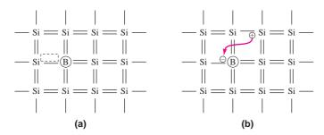
**Figure 1.7** (a) Two-dimensional representation of a silicon lattice doped with a boron atom showing the vacant covalent bond position, (b) the resulting negatively charged boron ion after it has accepted an electron from the valence band. A positively charged hole is created.
