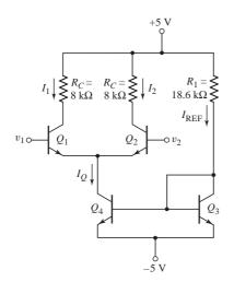
Figure 11.17 BJT differential amplifier for Example 11.6
