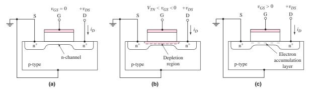
**Figure 3.14** Cross section of an n-channel depletion mode MOSFET for: (a)  $v_{GS} = 0$ , (b)  $v_{GS} < 0$ , and (c)  $v_{GS} > 0$
