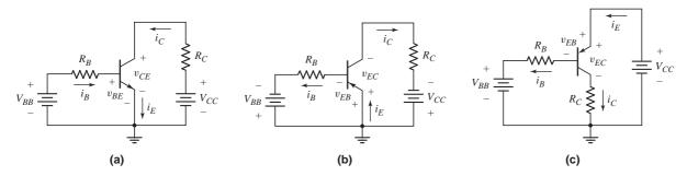
**Figure 5.10** Common-emitter circuits: (a) with an npn transistor, (b) with a pnp transistor, and (c) with a pnp transistor biased with a positive voltage source
