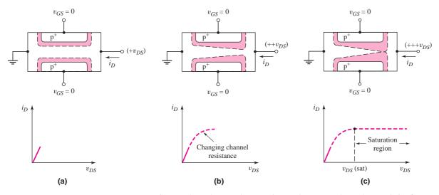
**Figure 3.56** Gate-to-channel space-charge regions and current–voltage characteristics for zero gate voltage and for: (a) a small drain voltage, (b) a larger drain voltage, and (c) a drain voltage that achieves pinchoff at the drain terminal
