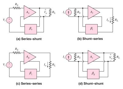
Figure 12.5 Basic feedback connections
