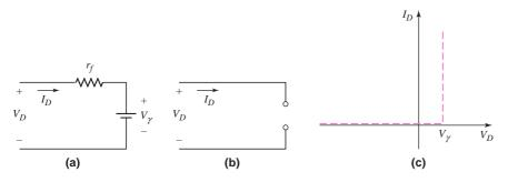
**Figure 1.31** The diode piecewise equivalent circuit (a) in the "on" condition when  $V_D \ge V_{\gamma}$ , (b) in the "off" condition when  $V_D < V_{\gamma}$ , and (c) piecewise linear approximation when  $r_f = 0$ . When  $r_f = 0$ , the voltage across the diode is a constant at  $V_D = V_{\gamma}$  when the diode is conducting.
