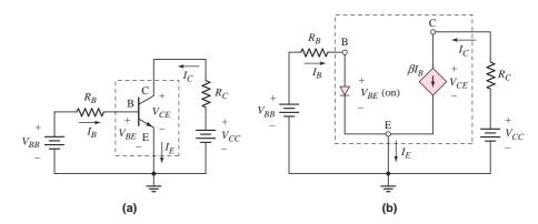
**Figure 5.19** (a) Common-emitter circuit with npn transistor and (b) dc equivalent circuit. Transistor equivalent circuit is shown within the dotted lines with piecewise linear transistor parameters.
