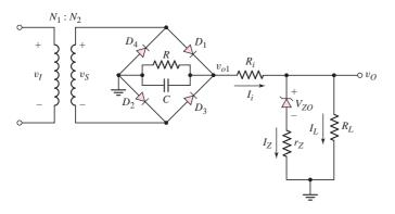
Figure 2.48 DC power supply circuit for design application
