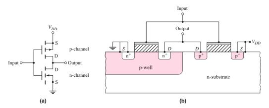
Figure 16.22 Simplified cross section, CMOS inverter
