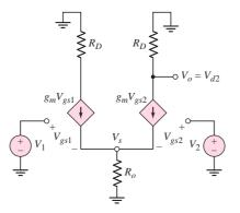
Figure 11.23 Small-signal equivalent circuit, MOSFET differential amplifier
