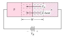
**Figure 1.13** A pn junction with an applied reverse-bias voltage, showing the direction of the electric field induced by  $V_R$  and the direction of the original space-charge electric field. Both electric fields are in the same direction, resulting in a larger net electric field and a larger barrier between the p- and n-regions.
