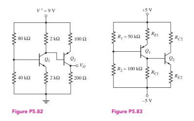
5.83 (a) For the transistors in the circuit shown in Figure P5.83, the parameters are:  $\beta = 100$  and  $V_{BE}(\text{on}) = V_{EB}(\text{on}) = 0.7$  V. Determine  $R_{C1}$ ,  $R_{E1}$ ,  $R_{C2}$ , and  $R_{E2}$  such that  $I_{C1} = I_{C2} = 0.8$  mA,  $V_{ECQ1} = 3.5$  V, and  $V_{CEQ2} = 4.0$  V. (b) Correlate the results of part (a) with a computer simulation.
