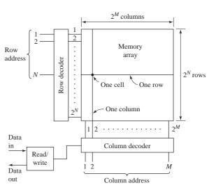
Figure 16.70 Schematic of a basic memory configuration
