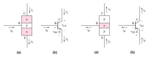
**Figure 5.8** npn bipolar transistor: (a) simple block diagram and (b) circuit symbol. Arrow is on the emitter terminal and indicates the direction of emitter current (out of emitter terminal for the npn device).
