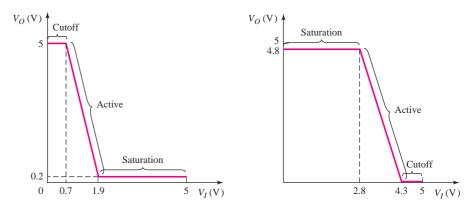
**Figure 5.28** Voltage transfer characteristics for (a) npn circuit in Figure 5.27(a) and (b) pnp circuit in Figure 5.27(b)
