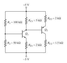
Figure 5.61 A multistage transistor circuit
