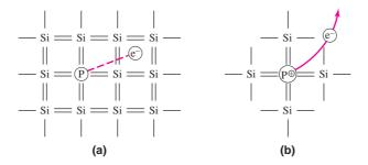
**Figure 1.6** (a) Two-dimensional representation of a silicon lattice doped with a phosphorus atom showing the fifth phosphorus valence electron, (b) the resulting positively charged phosphorus ion after the fifth valence electron has moved into the conduction band
