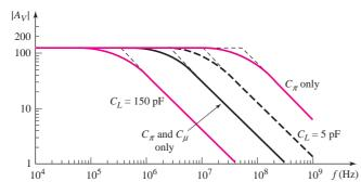
Figure 7.59 PSpice analysis results for common-emitter amplifier
