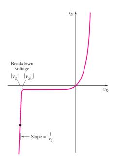
Figure 1.43 Diode I–V characteristics showing breakdown effects
