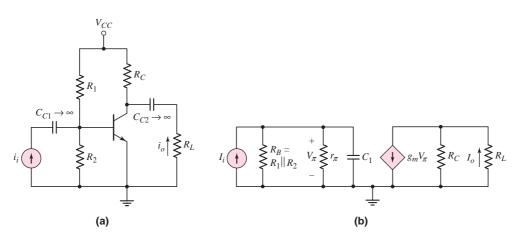
**Figure 12.48** (a) Single-stage common-emitter amplifier and (b) small-signal equivalent circuit, including input capacitance
