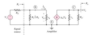
Figure 6.27 The small-signal equivalent circuit, assuming the coupling capacitor is a short circuit
