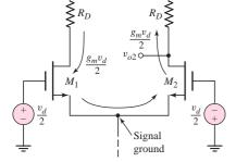
Figure 11.22 AC equivalent circuit, MOSFET differential amplifier
