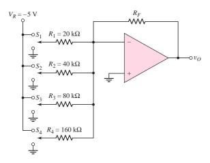
Figure 16.90 A 4-bit weighted-resistor D/A converter
