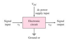
**Figure 6.1** Schematic of an electronic circuit with two input signals: the dc power supply input, and the signal input
