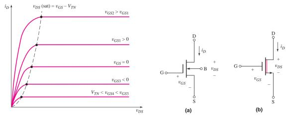
**Figure 3.15** Family of  $i_D$  versus  $v_{DS}$  curves for an n-channel depletion-mode MOSFET. Note again that the  $v_{DS}$ (sat) voltage is a single point on each curve.
