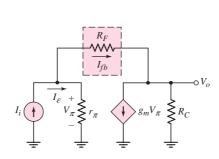
Figure 12.36 Small-signal equivalent circuit, discrete transistor shunt–shunt feedback configuration
