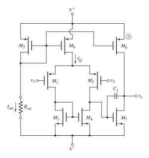
Figure 13.14 MC14573 CMOS op-amp equivalent circuit
