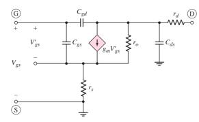
Figure 7.50 Equivalent circuit of the n-channel common-source MOSFET
