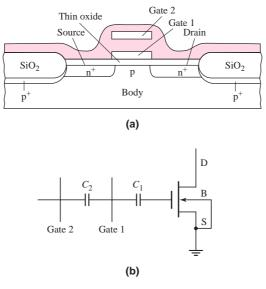
Figure 16.85 (a) Cross section of erasable programmable ROM; (b) equivalent circuit
