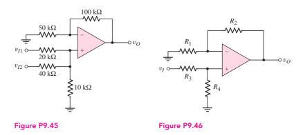
9.46 (a) Derive the expression for the closed-loop voltage gain  $A_v = v_O/v_I$  for the circuit shown in Figure P9.46. Assume an ideal op-amp. (b) Let
