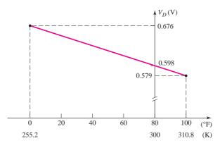
Figure 1.48 Diode voltage versus temperature
