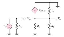
Figure 4.58 Small-signal equivalent circuit of JFET source-follower circuit
