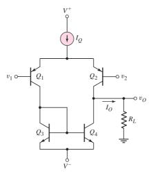
The circuit bias is  $I_Q = 0.2$  mA, and the transistor parameters are  $\beta = 100$  and  $V_A = 100$  V. (a) Determine  $I_0$  such that the dc currents in the diff-amp are balanced. (b) Find the open-circuit differential-mode voltage gain. (c) Determine the differential-mode voltage gain if a load resistance  $R_L = 250$  k $\Omega$  is connected to the output.
