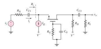
Figure 4.32 Common-gate circuit
