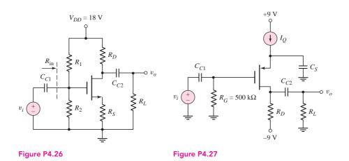
4.27 For the common-source amplifier shown in Figure P4.27, the transistor parameters are  $V_{TP} = -1.2$  V,  $K_p = 2 \text{ mA/V}^2$ , and  $\lambda = 0.03 \text{ V}^{-1}$ . The
