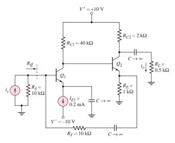
the small-signal parameters for  $Q_1$  and  $Q_2$ . (b) Using nodal analysis, determine the small-signal closed-loop current gain  $A_{if} = i_o/i_s$ . (c) Using nodal analysis, find the input resistance  $R_{if}$ .
