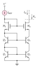
Figure 11.42 BiCMOS double cascode constant-current source
