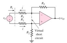
Figure 9.25 Circuit for measuring differential input resistance of op-amp difference amplifier
