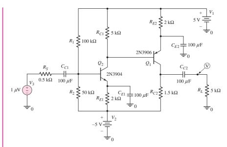
Figure 6.68 PSpice circuit schematic for Example 6.15
