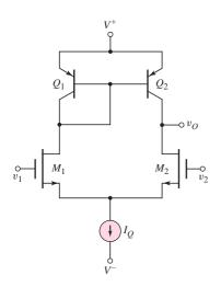
Figure 11.44 Basic BiCMOS differential amplifier
