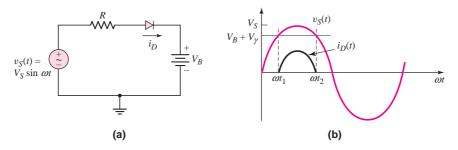
Figure 2.4 (a) Half-wave rectifier used as a battery charger; (b) input voltage and diode current waveforms
