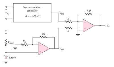
Figure 9.49 The output voltage  $V_{AT}$  applied to an instrumentation amplifier, an offset voltage generated by a Zener diode and a noninverting amplifier, and the final output voltage obtained from a summing amplifier
