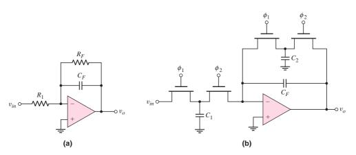
Figure 15.13 (a) One-pole low-pass filter and (b) equivalent switched-capacitor circuit
