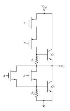
Figure 17.37 Two-input BiCMOS NOR circuit
