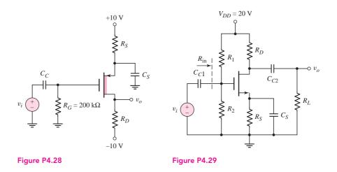
\*D4.29 Design a common-source amplifier, such as that in Figure P4.29, to achieve a small-signal voltage gain of at least  $A_v = v_o/v_i = -10$  for  $R_L = 20 \text{ k}\Omega$ and  $R_{\text{in}} = 200 \text{ k}\Omega$ . Assume the *Q*-point is chosen at  $I_{DQ} = 1$  mA and  $V_{DSQ} = 10$  V. Let  $V_{TN} = 2$  V, and  $\lambda = 0$ .
