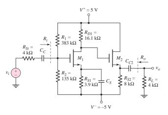
Figure 4.49 Common-source amplifier in cascade with source follower
