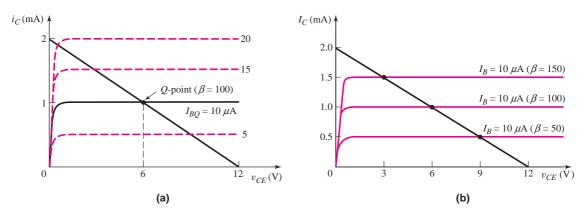
**Figure 5.52** (a) Transistor characteristics and load line for the circuit in Figure 5.51 used in Design Example 5.14; (b) load line and changes in the *Q*-point for  $\beta = 50$ , 100, and 150. (Note that the base current scale changes compared to the collector current scale.)
