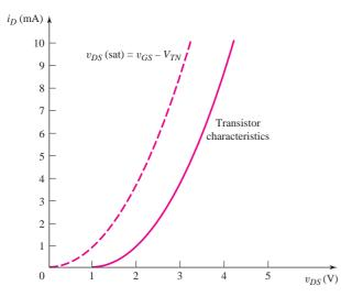
Figure 3.35 Current-voltage characteristic of an enhancement load device
