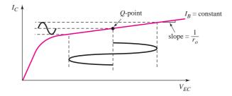
Figure 11.27 Current–voltage characteristic of active load device
