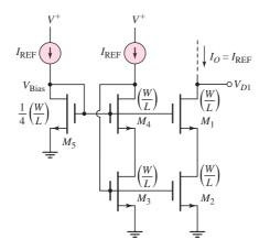
Figure 10.21 A wide-swing MOSFET cascode current mirror
