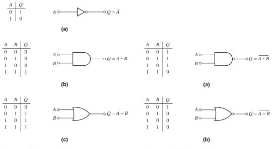
**Figure PR3.1** Truth tables, logic gate symbols, and Boolean expressions: (a) NOT function, (b) AND function, and (c) OR function
