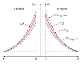
**Figure 1.37** Change in minority carrier stored charge with a time-varying voltage superimposed on a dc quiescent diode voltage. The change in stored charge leads to a diode diffusion capacitance.
