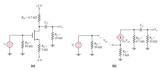
Figure 7.22 (a) Common-source circuit with output coupling capacitor and (b) small-signal equivalent circuit
