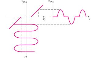
Figure 8.20 Voltage transfer characteristics of basic complementary push–pull output stage
