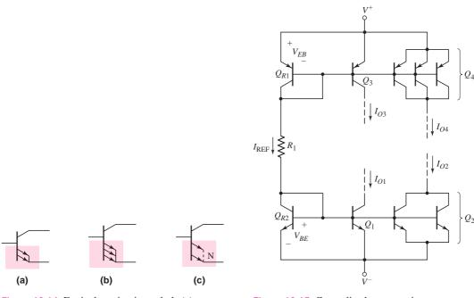
**Figure 10.14** Equivalent circuit symbols (a) two transistors in parallel, (b) three transistors in parallel, and (c) *N* transistors in parallel
