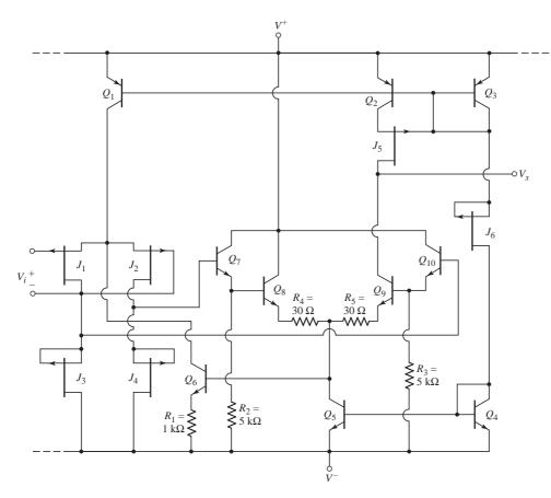
Figure 13.25 Equivalent circuit, LF155 BiFET op-amp input stages
