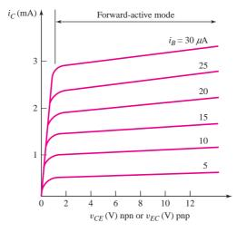
Figure 5.13 Transistor current-voltage characteristics of the common-emitter circuit
