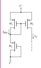
10.46 Consider the basic two-transistor NMOS current source in Figure 10.16. The circuit parameters are  $V^+ = +5$  V,  $V^- = -5$  V, and  $I_{\text{REF}} = 250 \ \mu\text{A}$ . The transistor parameters are  $V_{TN} = 1$  V,  $k'_n = 80 \ \mu\text{A/V}^2$ , and  $\lambda = 0.02 \ \text{V}^{-1}$ . (a) For  $(W/L)_1 = (W/L)_2 = 3$ , find  $I_O$  for (i)  $V_{DS2} = 3$  V, (ii)  $V_{DS2} = 4.5$  V, and (iii)  $V_{DS2} = 6$  V. (b) Repeat part (a) for  $(W/L)_1 = 3$  and  $(W/L)_2 = 4.5$ .
