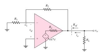
Figure 14.6 Equivalent circuit for calculating closed-loop output resistance
