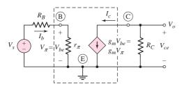
**Figure 6.11** The small-signal equivalent circuit of the common-emitter circuit shown in Figure 6.3. The small-signal hybrid- $\pi$  model of the npn bipolar transistor is shown within the dotted lines.
