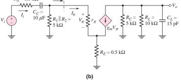
**Figure 7.26** (a) Circuit with both a coupling and a load capacitor and (b) small-signal equivalent circuit
