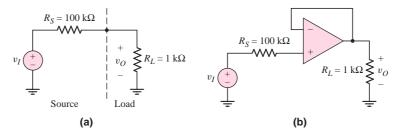
**Figure 9.18** (a) Source with a 100 k $\Omega$  output resistance driving a 1 k $\Omega$  load and (b) source with a 100 k $\Omega$  output resistance, voltage follower, and 1 k $\Omega$  load
