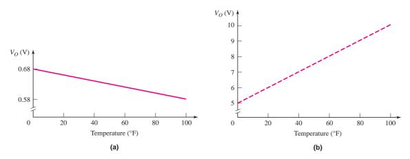
Figure 5.65 (a) Diode voltage versus temperature and (b) circuit output voltage versus temperature
