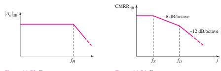
Figure 11.53 Frequency response of differential-mode gain
