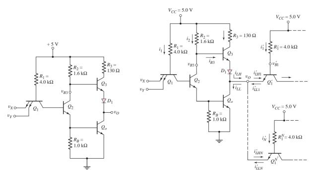
Figure 17.25 TTL circuit with totem-pole output stage
