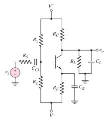
Figure 7.56 Common-emitter amplifier
