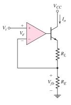
Figure 12.27 Example of an op-amp series–series feedback circuit
