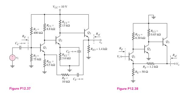
\*12.38 The circuit shown in Figure P12.38 is an ac equivalent circuit of a feedback amplifier. The transistor parameters are  $h_{FE} = 100$  and  $V_A = \infty$ . The quiescent collector currents are  $I_{C1} = 14.3$  mA,  $I_{C2} = 4.62$  mA, and  $I_{C3} =$
