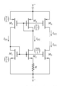
Figure 10.22 Bias-independent MOSFET current mirror
