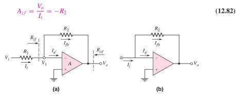
**Figure 12.33** (a) The basic inverting op-amp circuit and (b) the circuit showing the shunt input connection
