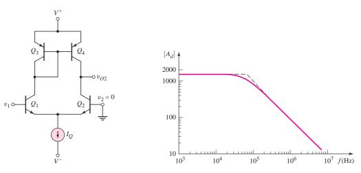
Figure 11.57 BJT diff-amp with active load and single-sided input
