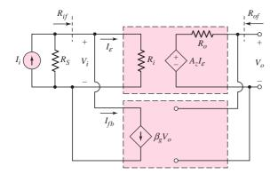
Figure 12.14 Ideal shunt-shunt feedback topology
