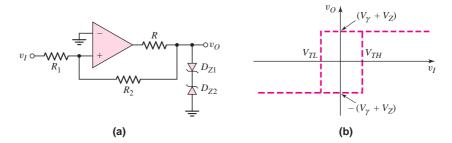
Figure 15.33 (a) Schmitt trigger with Zener diode limiters and (b) voltage transfer characteristics
