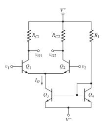
$I_{E1} = I_{S1}e^{V_{BE1}/V_T}$  and  $I_{E2} = I_{S2}e^{V_{BE2}/V_T}$ . (a) If  $v_1 = v_2 = 0$  and  $I_{S1} = I_{S2} = 3 \times 10^{-15}$  A, determine  $(v_{O1} - v_{O2})$  for (i)  $R_{C1} = R_{C2} = 7.5$  k $\Omega$  and (ii)  $R_{C1} = 7.4$  k $\Omega$ ,  $R_{C2} = 7.6$  k $\Omega$ . (b) Repeat part (a) for  $I_{S1} = 2.9 \times 10^{-15}$  A and  $I_{S2} = 3.1 \times 10^{-15}$  A.
