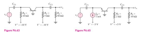
6.65 Consider the common-base circuit in Figure P6.65. The transistor has parameters  $\beta = 120$  and  $V_A = \infty$ . (a) Determine the quiescent  $V_{CEQ}$ . (b) Determine the small-signal voltage gain  $A_v = v_o/v_s$ .
