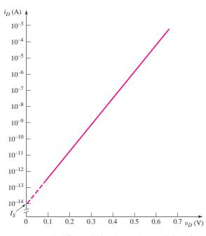
**Figure 1.18** Ideal forward-biased *I*–*V* characteristics of a pn junction diode, with the current plotted an a log scale for  $I_S = 10^{-14}$  A and n = 1. The diode current increases approximately one order of magnitude for every 60-mV increase in diode voltage.
