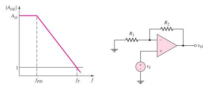
Figure 14.8 Bode plot, open-loop gain magnitude
