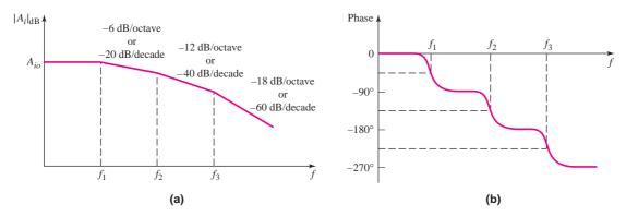
Figure 12.53 Bode plots of three-stage amplifier gain: (a) magnitude and (b) phase
