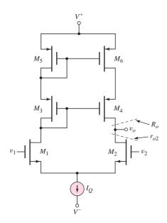
Figure 11.36 MOSFET diff-amp with cascode active load
