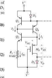
Figure 13.22 Bias circuit, CA3140 BiCMOS op-amp
