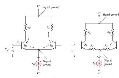
**Figure 11.14** BJT differential amplifier with differential-mode input signal, showing differential input resistance
