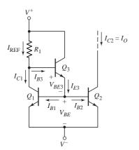
Figure 10.5 Basic three-transistor current source
