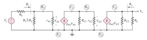
Figure 6.67 Small-signal equivalent circuit of the cascade circuit shown in Figure 6.66
