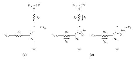
Figure 5.46 A bipolar (a) inverter circuit and (b) NOR logic gate
