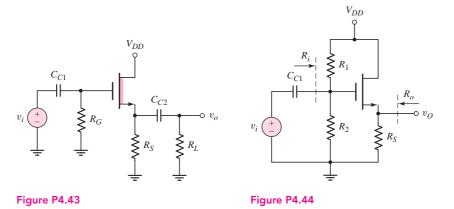
4.44 The transistor in the circuit in Figure P4.44 has parameters  $V_{TN} = 0.4$  V,  $K_n = 0.5 \text{ mA/V}^2$ , and  $\lambda = 0$ . The circuit parameters are  $V_{DD} = 3$  V and  $R_i = 300 \text{ k}\Omega$ . (a) Design the circuit such that  $I_{DQ} = 0.25$  mA and  $V_{DSQ} = 1.5$  V. (b) Determine the small-signal voltage gain and the output resistance  $R_{\rho}$ .
