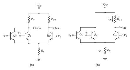
Figure 17.9 (a) Basic ECL OR/NOR logic gate and (b) modified ECL logic gate
