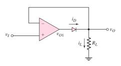
Figure 9.33 Precision half-wave rectifier circuit
