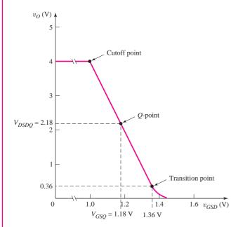
Figure 4.41 Voltage transfer characteristics and *Q*-point of NMOS amplifier with enhancement load, for Example 4.11
