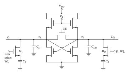
Figure 16.82 Sense amplifier configuration for dynamic RAM cell
