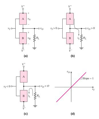
**Figure 8.18** (a) Idealized class-B output stage with complementary pair, A and B, of electronic devices; (b) device A turns on for  $v_I > 0$ , supplying current to the load; (c) device B turns on for  $v_I < 0$ , sinking current from the load; (d) ideal voltage transfer characteristics
