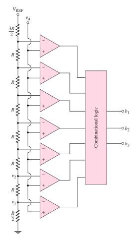
Figure 16.93 A 3-bit flash or parallel A/D converter
