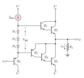
Figure 8.36 Class-AB output stage with Darlington pairs
