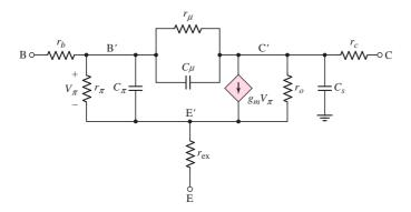
**Figure 7.37** Hybrid- $\pi$  equivalent circuit
