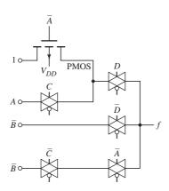
Figure 16.59 CMOS pass logic network
