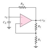
Figure 15.35 Schmitt trigger oscillator
