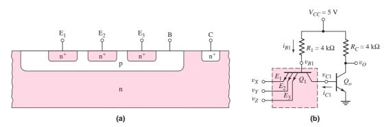
**Figure 17.22** (a) Simplified cross section of three-emitter transistor and (b) TTL circuit with three-emitter input transistor
