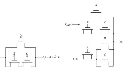
Figure 16.54 NMOS pass logic network with a potential problem
