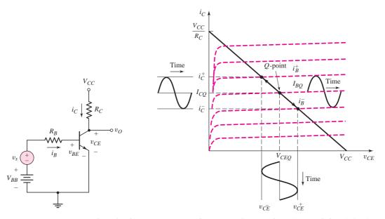
Figure 6.3 A common-emitter circuit with a time-varying signal source in series with the base dc source
