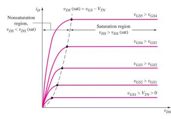
**Figure 3.10** Family of  $i_D$  versus  $v_{DS}$  curves for an n-channel enhancement-mode MOSFET. Note that the  $v_{DS}(\text{sat})$  voltage is a single point on each of the curves. This point denotes the transition between the nonsaturation region and the saturation region
