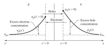
**Figure 1.16** Steady-state minority carrier concentrations in a pn junction under forward bias. The gradients in the minority carrier concentrations generate diffusion currents in the device.
