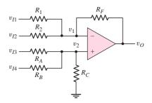
Figure 9.40 Generalized op-amp summing amplifier
