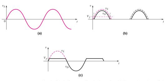
Figure 2.3 Signals of the half-wave rectifier circuit: (a) sinusoidal input voltage, (b) rectified output voltage, and (c) diode voltage
