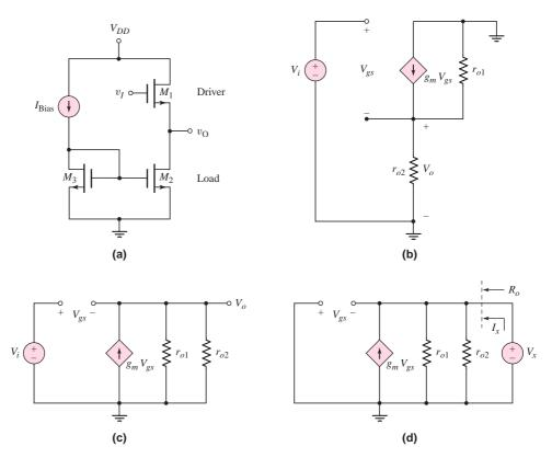
**Figure 4.47** (a) All NMOS source-follower circuit, (b) small-signal equivalent circuit, (c) reconfiguration of small-signal equivalent circuit, and (d) small-signal equivalent circuit for determining the output resistance
