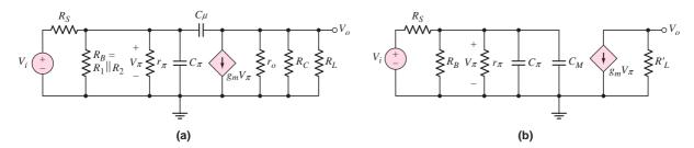
**Figure 7.57** (a) High-frequency equivalent circuit of common-emitter amplifier; (b) high-frequency equivalent circuit of common-emitter amplifier, including the Miller capacitance
