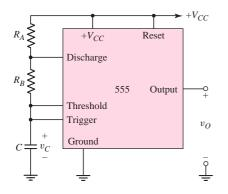
Figure 15.41 Astable multivibrator 555 circuit
