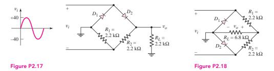
\*2.18 (a) Sketch  $v_o$  versus time for the circuit in Figure P2.18. The input is a sine wave given by  $v_i = 10 \sin \omega t$  V. Assume  $V_{\gamma} = 0$ . (b) Determine the rms value of the output voltage.
