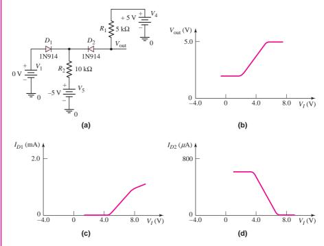
**Figure 2.37** (a) PSpice circuit schematic; (b) output voltage; (c) current in diode 1, and (d) current in diode 2 for the diode circuit in Example 2.9
