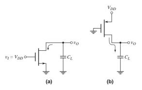
Figure 16.35 (a) Effective CMOS inverter in pull-down mode and (b) effective CMOS inverter in pull-up mode
