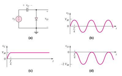
**Figure 2.27** Action of a diode clamper circuit: (a) a typical diode clamper circuit, (b) the sinusoidal input signal, (c) the capacitor voltage, and (d) the output voltage
