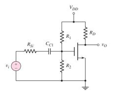
Figure 4.14 Common-source circuit with voltage divider biasing and coupling capacitor
