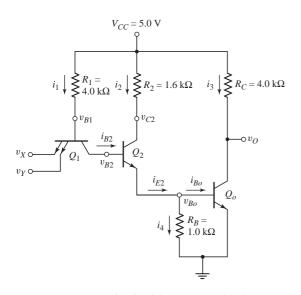
Figure 17.24 TTL circuit with currents and voltages
