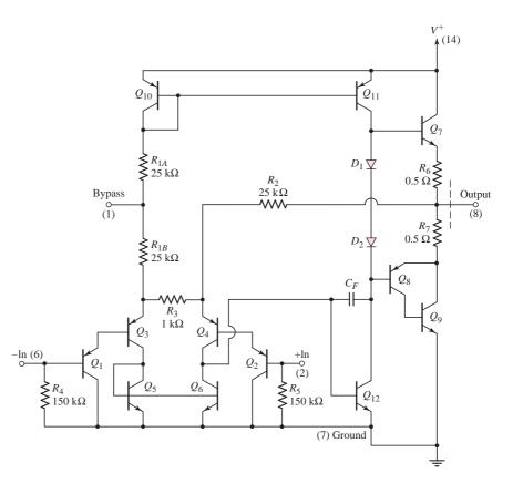
Figure 15.42 The LM380 power amplifier
