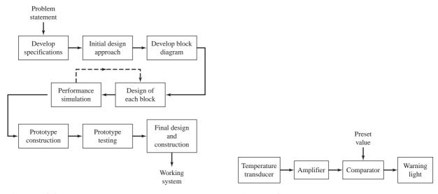
Figure PR2.3 Flowchart of the design process
