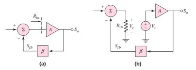
**Figure 12.43** (a) Basic feedback network, showing amplifier input resistance and (b) feedback network after the loop is broken, showing test voltage and load resistance
