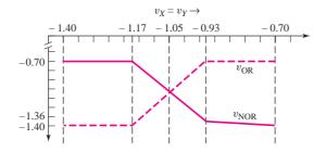
Figure 17.8 ECL OR/NOR logic gate voltage transfer characteristics
