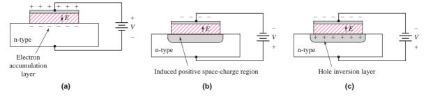
**Figure 3.4** The MOS capacitor with n-type substrate: (a) effect of a positive gate bias and the formation of an electron accumulation layer, (b) the MOS capacitor with an induced space-charge region due to a moderate negative gate bias, and (c) the MOS capacitor with an induced space-charge region and hole inversion layer due to a larger negative gate bias
