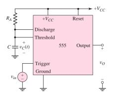
Figure 15.40 The 555 circuit connected as a monostable multivibrator
