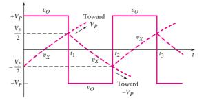
Figure 15.36 Output voltage and capacitor voltage versus time for Schmitt trigger oscillator
