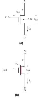
Figure 3.18 The p-channel depletion mode MOSFET: (a) conventional circuit symbol and (b) simplified circuit symbol
