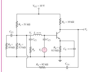
Figure 12.45 Feedback circuit with the loop effectively broken, for determining the loop gain from a computer analysis
