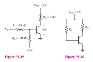
D5.40 (a) The circuit shown in Figure P5.40 is to be designed such that  $I_{CQ} = 0.5 \text{ mA}$  and  $V_{CEQ} = 2.5 \text{ V}$ . Assume  $\beta = 120$ . Sketch the load line and plot the *Q*-point. (b) Pick standard values of resistors that are close to the designed values. Assume that the standard resistor values vary by  $\pm 10$
