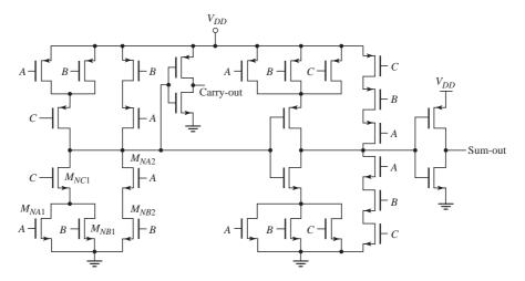
Figure 16.69 Transistor configuration of the CMOS one-bit full adder
