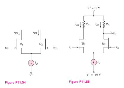
11.55 A JFET differential amplifier is shown in Figure P11.55. The transistor parameters are:  $V_P = -4 \text{ V}$ ,  $I_{DSS} = 2 \text{ mA}$ , and  $\lambda = 0$ . (a) Find  $R_D$  and  $I_Q$  such that  $I_{D1} = I_{D2} = 0.5 \text{ mA}$  and  $v_{o2} = 7 \text{ V}$  when  $v_1 = v_2 = 0$ .
