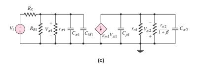
**Figure 7.66** (a) High-frequency equivalent circuit of cascode configuration, (b) rearranged high-frequency equivalent circuit, and (c) variation of the high-frequency circuit, including the Miller capacitance
