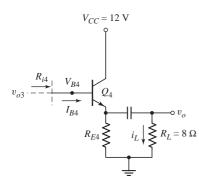
Figure 6.78 Output stage (emitter-follower) for design application
