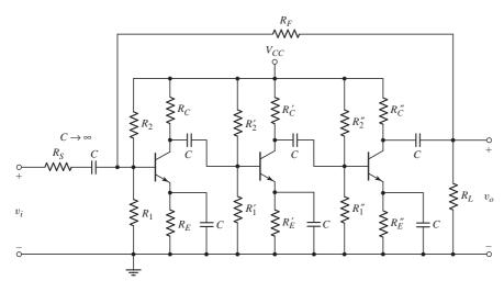
Figure 12.41 Example of multistage shunt-shunt feedback circuit
