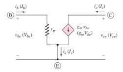
**Figure 6.9** A simplified small-signal hybrid- $\pi$  equivalent circuit for the npn transistor. The ac signal currents and voltages are shown. The phasor signals are shown in parentheses.
