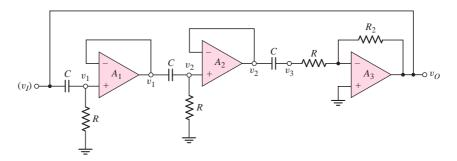
Figure 15.15 Phase-shift oscillator circuit with voltage-follower buffer stages
