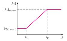
Figure 7.28 Bode plot of the voltage gain magnitude for the circuit with an emitter bypass capacitor
