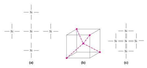
**Figure 1.1** Silicon atoms in a crystal matrix: (a) five noninteracting silicon atoms, each with four valence electrons, (b) the tetrahedral configuration, (c) a two-dimensional representation showing the covalent bonding
