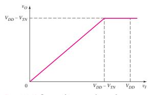
Figure 16.48 Output voltage versus input voltage characteristics of the NMOS transmission gate
