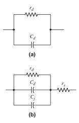
Figure 1.38 Small-signal equivalent circuit of the diode: (a) simplified version and (b) complete circuit
