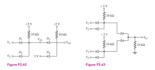
2.63 Determine the Boolean expression for  $V_0$  in terms of the four input voltages for the circuit in Figure P2.63 (Hint: A truth table might be helpful.)
