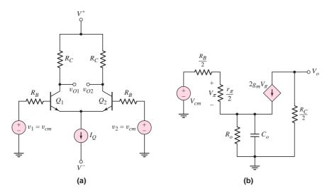
**Figure 11.51** (a) BJT differential amplifier with common-mode input signal and (b) small-signal equivalent circuit, common-mode configuration
