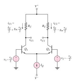
Figure 11.7 BJT differential amplifier with differential-mode input signal
