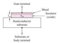
Figure 3.1 The basic MOS capacitor structure
