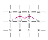
Figure 1.5 A two-dimensional representation of the silicon crystal showing the movement of the positively charged "empty state"
