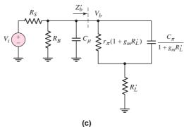
**Figure 7.69** (a) High-frequency equivalent circuit of emitter follower, (b) rearranged high-frequency equivalent circuit, and (c) high-frequency equivalent circuit with effective input base impedance
