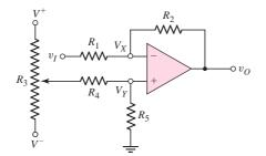
Figure 14.20 Offset voltage compensation circuit for inverting amplifier
