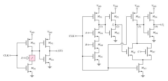
Figure 16.45 Generalized CMOS clocked logic circuit
