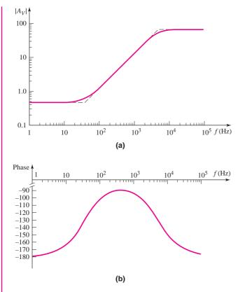
**Figure 7.29** PSpice analysis results for the circuit with an emitter bypass capacitor: (a) voltage gain magnitude response and (b) phase response
