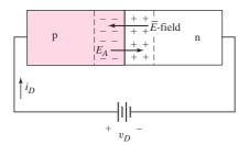
Figure 1.15 A pn junction with an applied forward-bias voltage showing the direction of the electric field induced by  $V_D$  and the direction of the original space-charge electric field. The two electric fields are in opposite directions resulting in a smaller net electric field and a smaller barrier between the p- and n-regions. The net electric field is always from the n- to the p-region.
