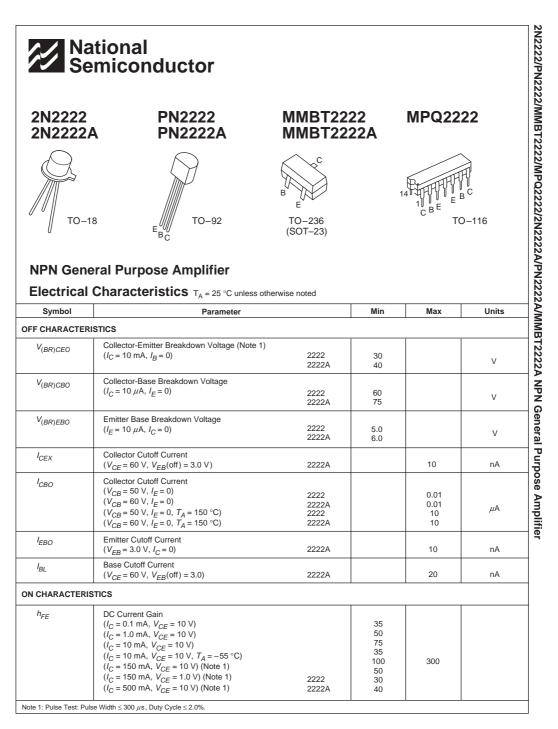
Figure 6.22 Basic data sheet for the 2N2222 bipolar transistor
