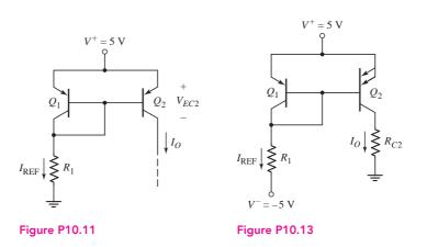
D10.13 Consider the pnp current source in Figure P10.13, with transistor parameters  $\beta = \infty$ ,  $V_A = \infty$ , and  $V_{EB}(\text{on}) = 0.7$  V. (a) Design the circuit such that  $I_{\text{REF}} = 1$  mA. (b) What is the value of  $I_O$ ? (c) What is the maximum value of  $R_{C2}$  such that  $Q_2$  remains biased in the forward-active mode?
