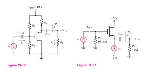
4.37 Consider the source follower circuit in Figure P4.37 with transistor parameters  $V_{TN} = 0.8 \text{ V}$ ,  $k'_n = 100 \,\mu\text{A/V}^2$ , W/L = 20, and  $\lambda = 0.02 \text{ V}^{-1}$ . (a) Let  $I_Q = 5 \text{ mA}$ . (i) Determine the small-signal voltage gain. (ii) Find the output resistance  $R_o$ . (b) Repeat part (a) for  $I_Q = 2 \text{ mA}$ .
