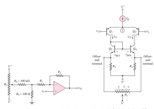
Figure 14.21 Offset voltage compensation circuit for noninverting amplifier
