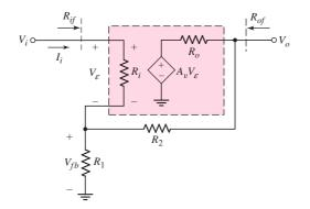
Figure 12.17 Equivalent circuit, op-amp series-shunt feedback configuration
