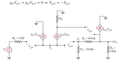
Figure 12.63 Small-signal equivalent circuit of the MOSFET feedback circuit for the design application
