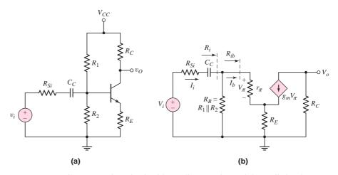
**Figure 7.21** (a) Common-emitter circuit with coupling capacitor and (b) small-signal equivalent circuit
