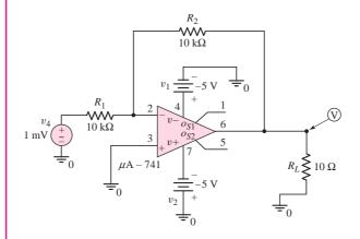
Figure 14.7 Circuit using 741 op-amp to measure output resistance
