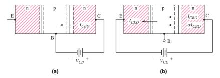
Figure 5.15 Block diagram of an npn transistor in an (a) open-emitter configuration showing the junction leakage current  $I_{CBO}$  and (b) open-base configuration showing the leakage current  $I_{CEO}$
