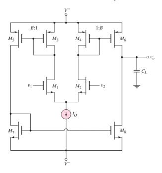
Figure 13.18 CMOS current-mirror op-amp
