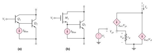
**Figure 11.38** (a) Bipolar Darlington pair configuration and (b) BiCMOS Darlington pair configuration
