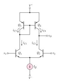
Figure 14.18 Basic bipolar diff-amp with active load
