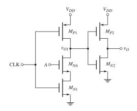
Figure 16.43 Simple clocked CMOS logic circuit
