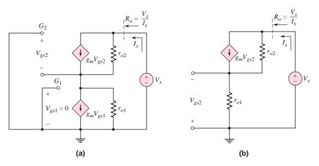
**Figure 10.26** (a) Equivalent circuit, using phasor notation, of the JFET cascode current source for determining output resistance and (b) final configuration
