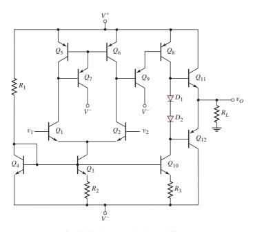
Figure 13.2 A simple bipolar operational amplifier
