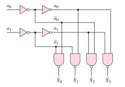
Figure 16.72 Simplified decoder with two-bit input
