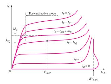
Figure 5.18 Common-emitter characteristics showing breakdown effects
