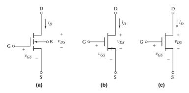
**Figure 3.12** The n-channel enhancement-mode MOSFET: (a) conventional circuit symbol, (b) circuit symbol that will be used in this text, and (c) a simplified circuit symbol used in more advanced texts
