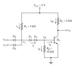
Figure 17.20 Basic diode-transistor logic gate
