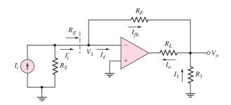
Figure 12.20 Example of an op-amp shunt-series feedback circuit
