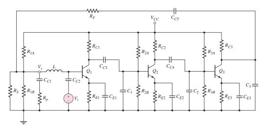
Figure 12.46 The ac equivalent circuit of three-stage feedback amplifier, including load capacitors
