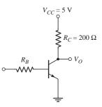
5.46 Consider the circuit in Figure P5.46. For the transistor,  $\beta = 50$ . Find  $I_B$ ,  $I_C$ ,  $I_E$ , and  $V_O$  for (a)  $V_I = 0$ , (b)  $V_I = 2.5$  V, and (c)  $V_I = 5$  V.
