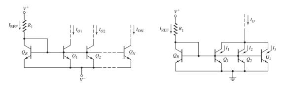
Figure 10.12 Multitransistor current mirror
