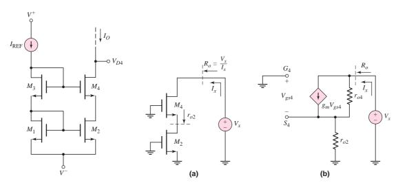
Figure 10.18 MOSFET cascode current mirror
