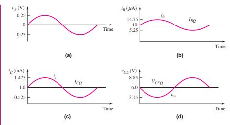
**Figure 6.12** The dc and ac signals in the common-emitter circuit: (a) input voltage signal, (b) input base current, (c) output collector current, and (d) output collector-emitter voltage. The ac output voltage is 180° out of phase with respect to the input voltage signal.
