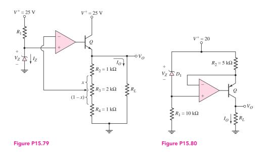
Zener voltage is  $V_{ZO} = 5.6$  V and the Zener resistance is  $r_z = 12 \Omega$ . (a) For  $I_Z = 12$  mA, find  $R_1$ . (b) Determine the range of output voltage as the potentiometer  $R_3$  is varied. (c) If the potentiometer is set such x = 1, determine the load regulation. Assume  $R_o$  of the op-amp is zero.
