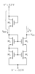
**Figure 10.42** MOSFET cascode current source circuit for design application
