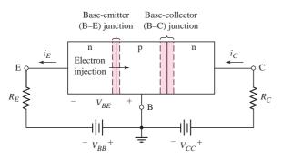
Figure 5.3 An npn bipolar transistor biased in the forward-active mode; base–emitter junction forward biased and base–collector junction reverse biased
