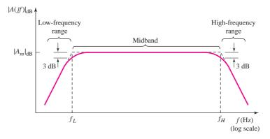
Figure 7.1 Amplifier gain versus frequency
