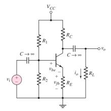
Figure 12.29 Example of a discrete transistor series—series feedback circuit
