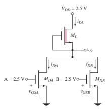
Figure 16.11 Two-input NMOS NOR logic gate with depletion load
