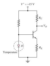
Figure 5.64 Design application circuit to measure output voltage of diode versus temperature
