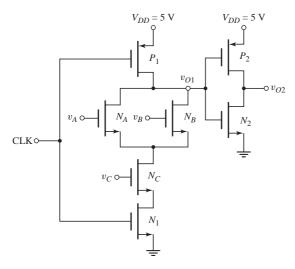
16.62 (a) For the circuit in Figure P16.62, make a table showing the state of each transistor ("on" or "off"), and determine the output voltages  $v_{O1}$ ,  $v_{O2}$ , and  $v_{O3}$  for the input logic states listed in the following table. Assume the input conditions are sequential in time from state 1 to state 6. (b) What logic function does the circuit implement?
