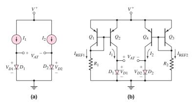
**Figure 9.48** (a) Two diodes biased with constant current sources. (b) The same circuit with the constant current sources implemented with transistor circuits.
