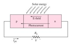
Figure 1.39 A pn junction solar cell connected to load
