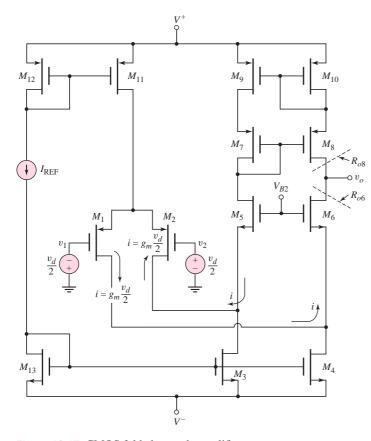
Figure 13.17 CMOS folded cascode amplifier
