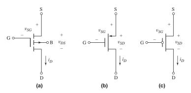
**Figure 3.13** The p-channel enhancement-mode MOSFET: (a) conventional circuit symbol, (b) circuit symbol that will be used in this text, and (c) a simplified circuit symbol used in more advanced texts
