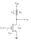
Figure 3.45 NMOS inverter circuit
