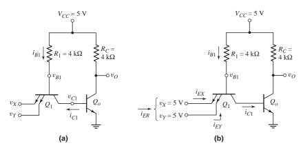
Figure 17.23 TTL circuit (a) with at least one input low and (b) with all inputs high
