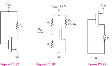
The transistor in Figure P3.28 has parameters  $V_{TN} = 0.4$  V,  $k'_n = 120$
