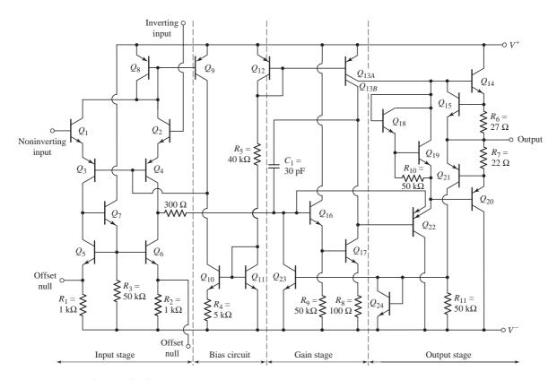
Figure 13.3 Equivalent circuit, 741 op-amp
