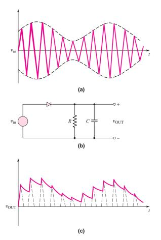
**Figure 2.13** The signals and circuit for demodulation of an amplitude-modulated signal. (a) The amplitude-modulated input signal. (b) The detector circuit. (c) The demodulated output signal.
