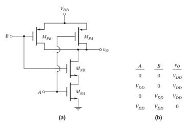
Figure 16.34 (a) Two-input CMOS NAND logic circuit and (b) truth table
