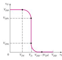
Figure 16.26 Complete voltage transfer characteristics, CMOS inverter
