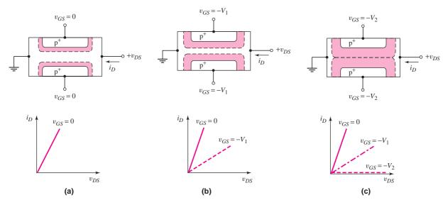
**Figure 3.55** Gate-to-channel space-charge regions and current–voltage characteristics for small drain-to-source voltages and for: (a) zero gate voltage, (b) small reverse-biased gate voltage, and (c) a gate voltage that achieves pinchoff
