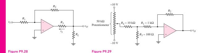
\*D9.29 Design the amplifier in Figure P9.29 such that the output voltage varies between  $\pm 10$  V as the wiper arm of the potentiometer changes from -10 V to +10 V. What is the purpose of including  $R_3$  and  $R_4$  instead of connecting  $R_1$  directly to the wiper arm?
