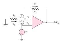
Figure 9.15 Noninverting op-amp circuit
