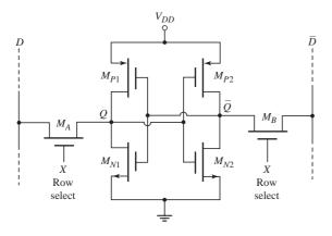
Figure 16.75 A CMOS static RAM cell
