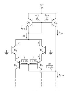
Figure 13.6 Expanded input stage, 741 op-amp, showing base currents
