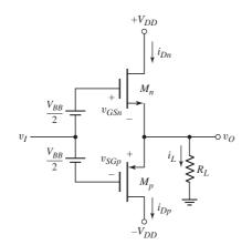
Figure 8.26 MOSFET class-AB output stage
