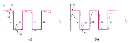
**Figure 7.20** Steady-state output response for a square-wave input response for (a) circuit in Figure 7.16 (coupling capacitor) and a large time constant, and (b) circuit in Figure 7.18 (load capacitor) and a short time constant
