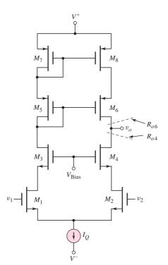
Figure 11.37 A MOSFET cascode diff-amp with a cascode active load
