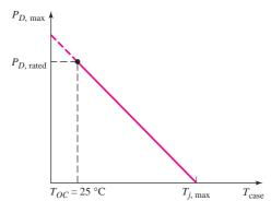
Figure 8.12 A power derating curve
