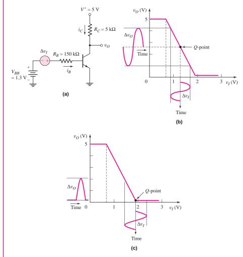
**Figure 5.50** (a) The inverter circuit with both a dc and an ac input signal; (b) the dc voltage transfer characteristics, *Q*-point, and sinusoidal input and output signals; (c) the transfer characteristics showing improper dc biasing
