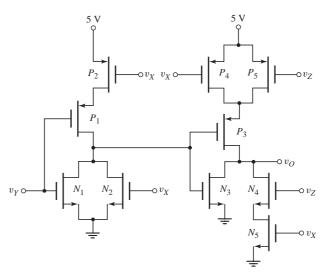
of part (b) and assuming  $v_A = v_B = 5$  V, determine  $v_C$  such that both  $N_3$  and  $P_3$  are biased in the saturation region. (State any assumptions you make.)
