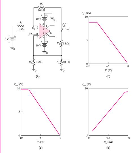
**Figure 9.23** (a) PSpice circuit schematic; (b) load current and (c) op-amp output voltage versus input voltage; (d) op-amp output voltage versus load resistance for  $v_1 = -5$  V
