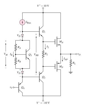
Figure 8.38 Output stage for design application
