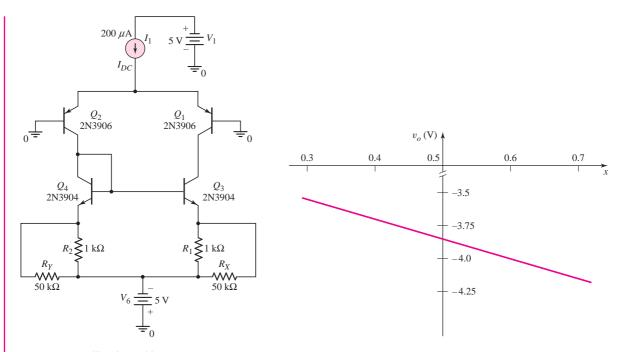
Figure 14.23 Circuit used in the computer simulation analysis for Example 14.12
