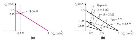
**Figure 1.32** Piecewise linear diode approximation superimposed on (a) load line for  $V_{PS} = 5 \text{ V}$ ,  $R = 2 \text{ k}\Omega$  and (b) several load lines. The Q-point of the diode changes when the load line changes.
