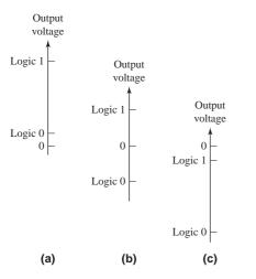
Figure PR3.4 Three possible output voltage combinations representing positive logic
