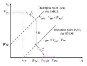
**Figure 16.25** Regions of the CMOS transfer characteristics indicating NMOS and PMOS transistor bias conditions. The NMOS device is biased in the saturation region in areas A and B and in the nonsaturation region in area C. The PMOS device is biased in the saturation region in areas B and C and in the nonsaturation region in area A.
