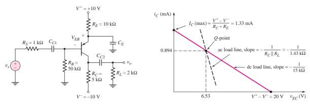
Figure 6.43 Circuit for Example 6.9
