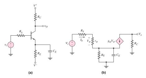
Figure 7.27 (a) Circuit with emitter bypass capacitor and (b) small-signal equivalent circuit
