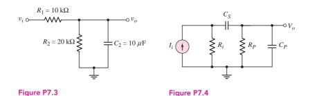
(a) Determine the open-circuit time constant associated with  $C_s$  and the short-circuit time constant associated with  $C_P$ . (b) Determine the corner frequencies and the magnitude of the transfer function  $T(s) = V_o(s)/I_i(s)$  at midband. (c) Sketch the Bode magnitude plot.
