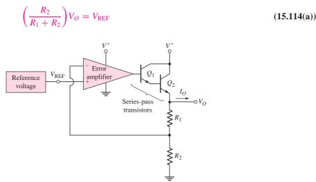
Figure 15.49 Basic series-pass voltage regulator
