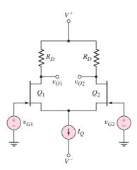
Figure 11.25 Basic JFET differential pair configuration
