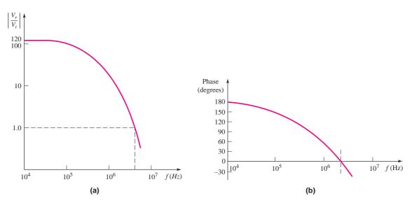
**Figure 12.47** (a) Bode plot of loop gain magnitude for three-stage feedback amplifier, from Example 12.17; (b) phase of the return signal for the three-stage amplifier
