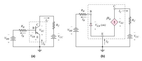
**Figure 5.21** (a) Common-emitter circuit with pnp transistor and (b) dc equivalent circuit. Transistor equivalent circuit is shown within the dotted lines with piecewise linear transistor parameters.
