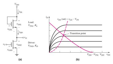
Figure 16.5 (a) NMOS inverter with saturated load and (b) driver transistor characteristics and load curve
