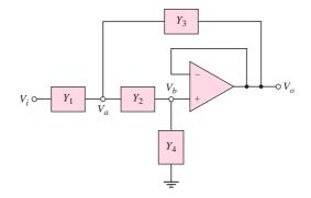
Figure 15.5 General two-pole active filter
