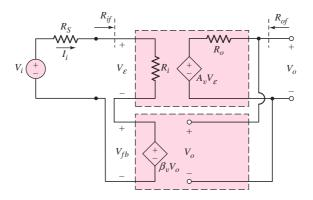
Figure 12.6 Ideal series-shunt feedback topology
