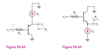
6.43 The circuit and transistor parameters for the ac equivalent circuit in Figure P6.43 are R<sub>S</sub> = 0.5 kΩ, β = 120, and V<sub>A</sub> = ∞. (a) Determine the required value of I<sub>Q</sub> to produce a small-signal output resistance of R<sub>o</sub> = 15 Ω. (b) Using the results of part (a), find the small-signal voltage gain if V<sub>A</sub> = 50 V.
