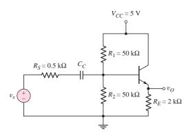
**Figure 6.49** Emitter-follower circuit. Output signal is at the emitter terminal with respect to ground.
