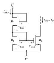
Figure 10.17 MOSFET current source
