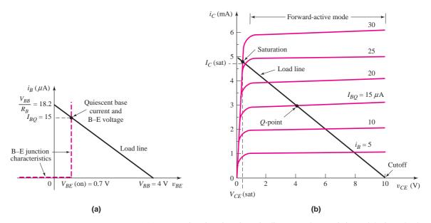
**Figure 5.23** (a) Base–emitter junction piecewise linear i-v characteristics and the input load line, and (b) common-emitter transistor characteristics and the collector–emitter load line showing the *Q*-point for the circuit shown in Example 5.3 (Figure 5.20)
