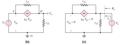
**Figure 4.48** (a) CMOS common-gate amplifier, (b) small-signal equivalent circuit, and (c) small-signal equivalent circuit for determining the output resistance
