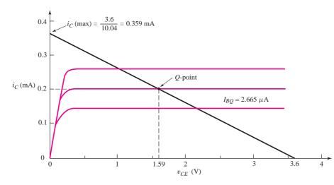
Figure 5.31 Load line and Q-point for the circuit shown in Figure 5.30 for Example 5.7
