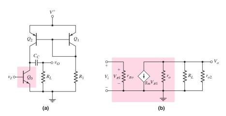
Figure 10.37 (a) Simple BJT amplifier with active load and load resistance and (b) smallsignal equivalent circuit
