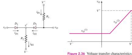
for the two-diode circuit in Figure 2.35
