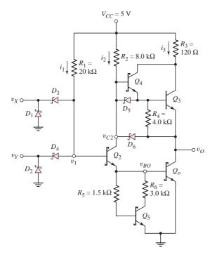
Figure 17.34 Low-power Schottky TTL NAND logic circuit
