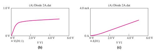
Figure 1.34 (a) PSpice circuit schematic, (b) diode voltage, and (c) diode current for Example 1.10
