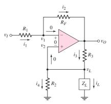
Figure 9.21 Simple voltage-to-current converter
