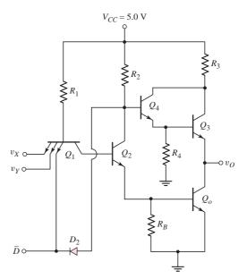
Figure 17.29 TTL circuit with tristate output stage
