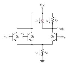
Figure 17.10 Modified ECL logic gate with Schottky diode
