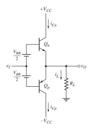
Figure 8.24 Bipolar class-AB output stage
