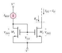
Figure 10.16 Basic two-transistor MOSFET current source
