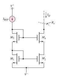
Figure 11.24 MOSFET cascode current source
