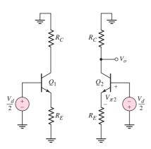
Figure 11.18 Differential half-circuits with emitter degeneration
